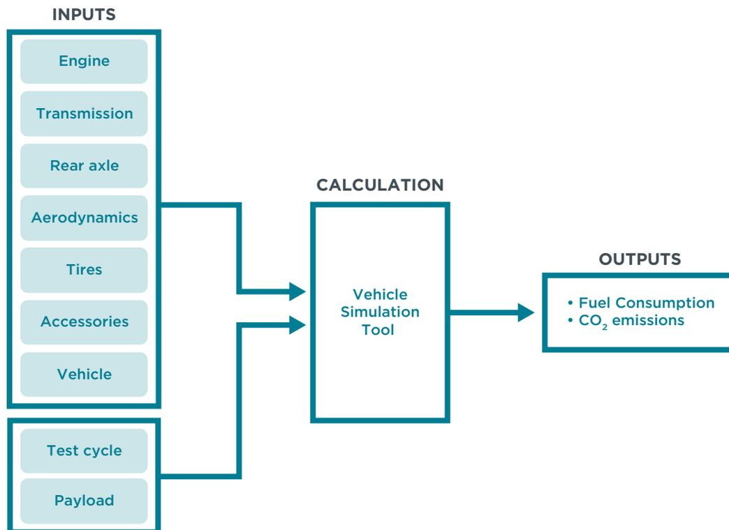
Figure 5. Vehicle simulation flowchart
