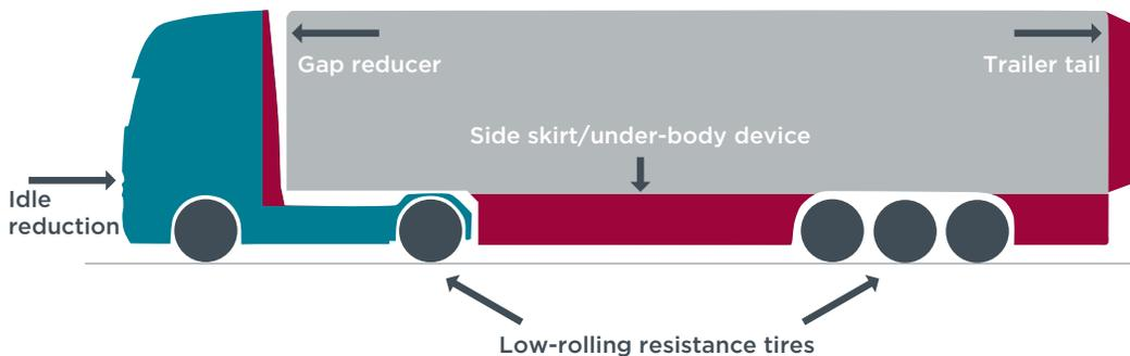
**Figure 3.** Available verified technology devices under SmartWay Program<sup>2</sup>
