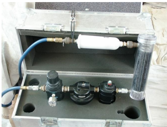
Figure A-3 Field Processing Unit for Purifying Dilution Air in Carrying Case
