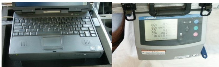
Figure A-4 Gas analyzer setup with continuous data logging system
