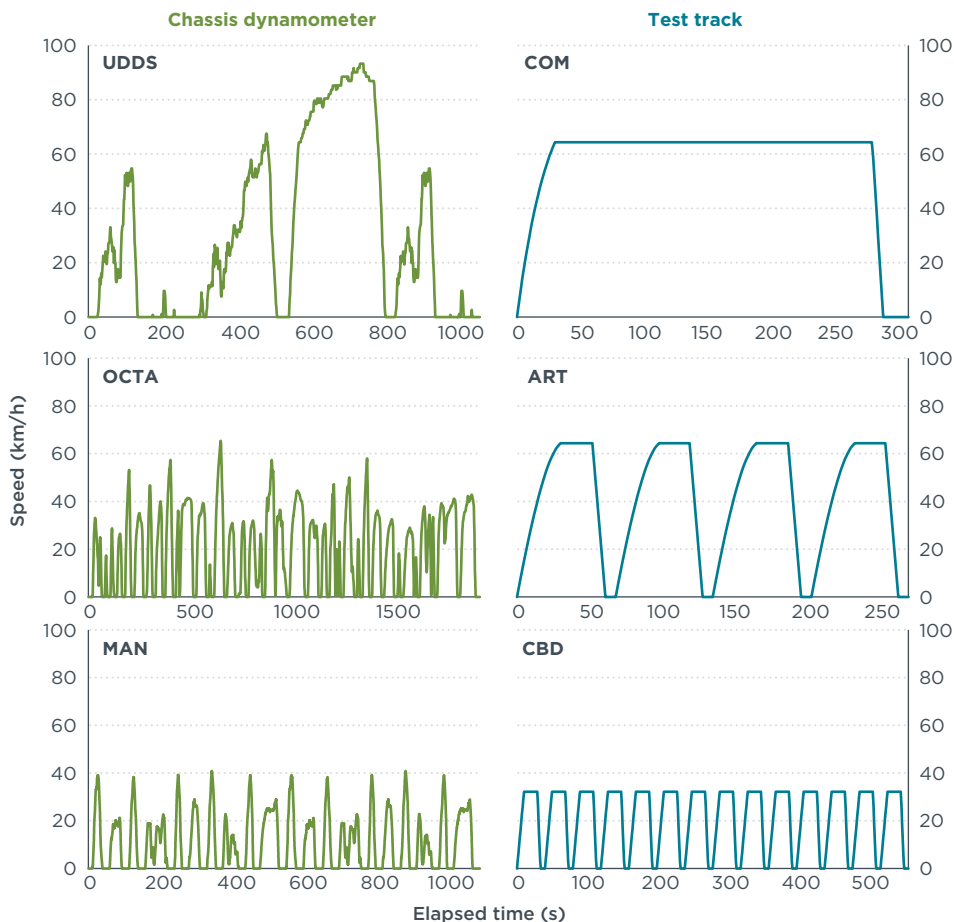
Figure 2. Speed-time traces for Altoona test program driving cycles. 9
