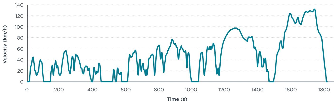
Figure 5. WLTP driving cycle (WLTC)
