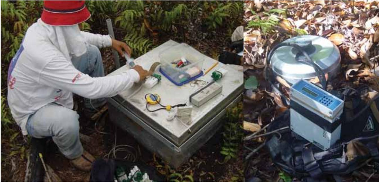
**Figure 7:** Closed chamber measurements being made in the field; large static chamber (left) and dynamic chamber and CO<sub>2</sub> analyzer (right; images: J. Jauhiainen).
