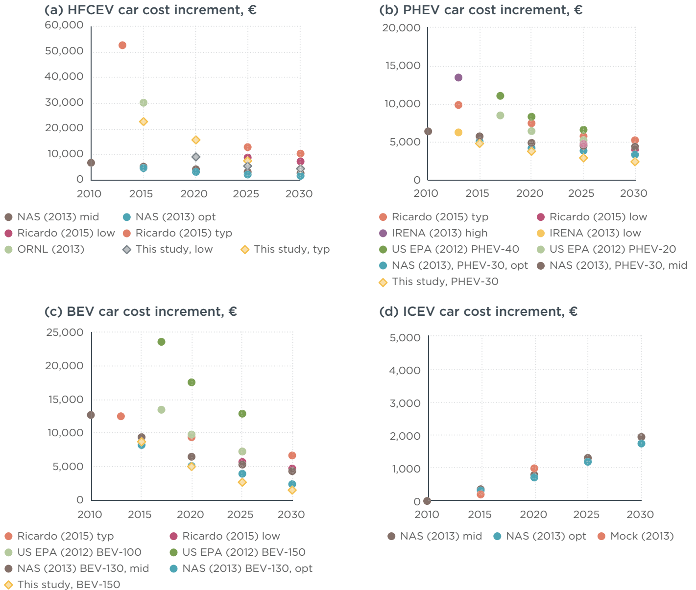
Figure 7. Estimated cost increment of EV power trains over a 2010 ICEV passenger car. Production scales can vary considerably between different studies. Own estimates for 2015 are based on an assumed ~50,000+ produced batteries and ~1,000 fuel cell systems; for 2030 ~500,000+ battery packs and ~50,000 (typical) to ~100,000 (low-cost) fuel cell systems are assumed.
