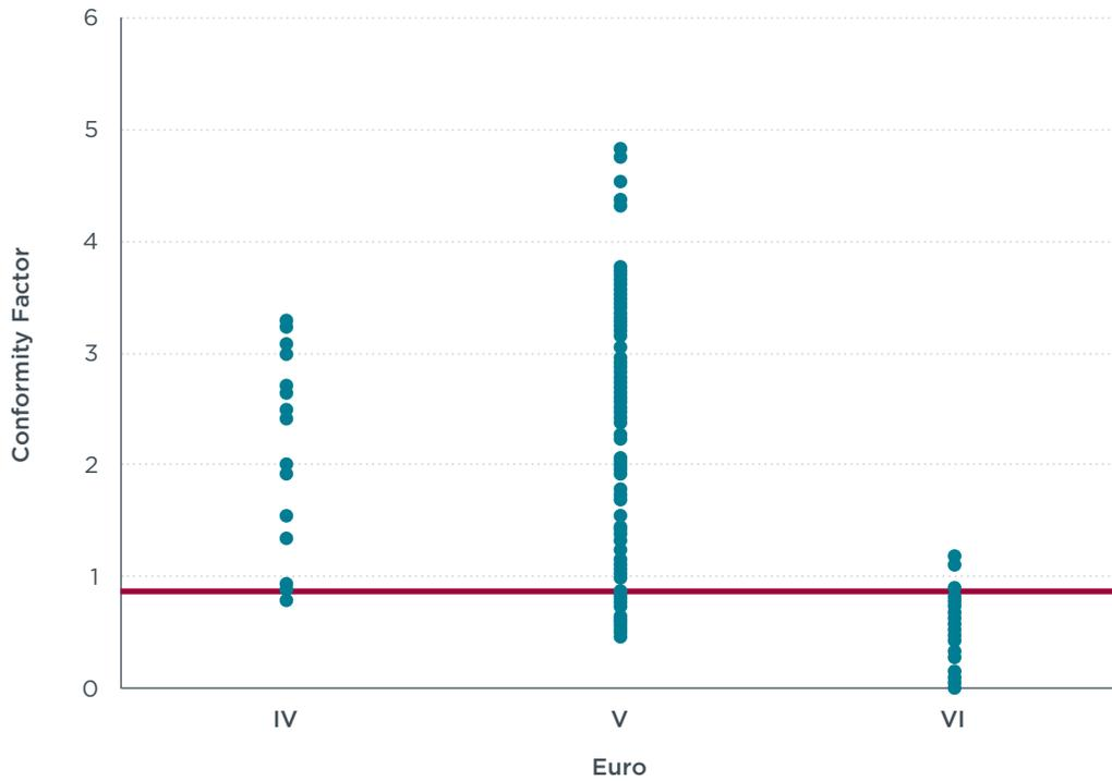
**Figure 4.** NO<sub>x</sub> emissions conformity factors for all tests plotted vs Euro level. Red line to indicate conformity factor of one.
