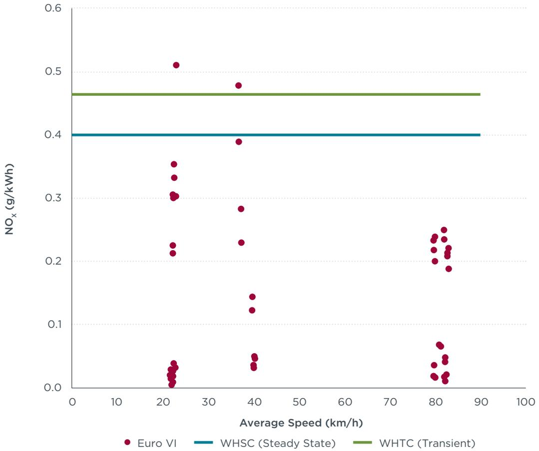
Figure 2. Euro VI NO<sub>x</sub> Emissions vs Average Speed for all Tests
