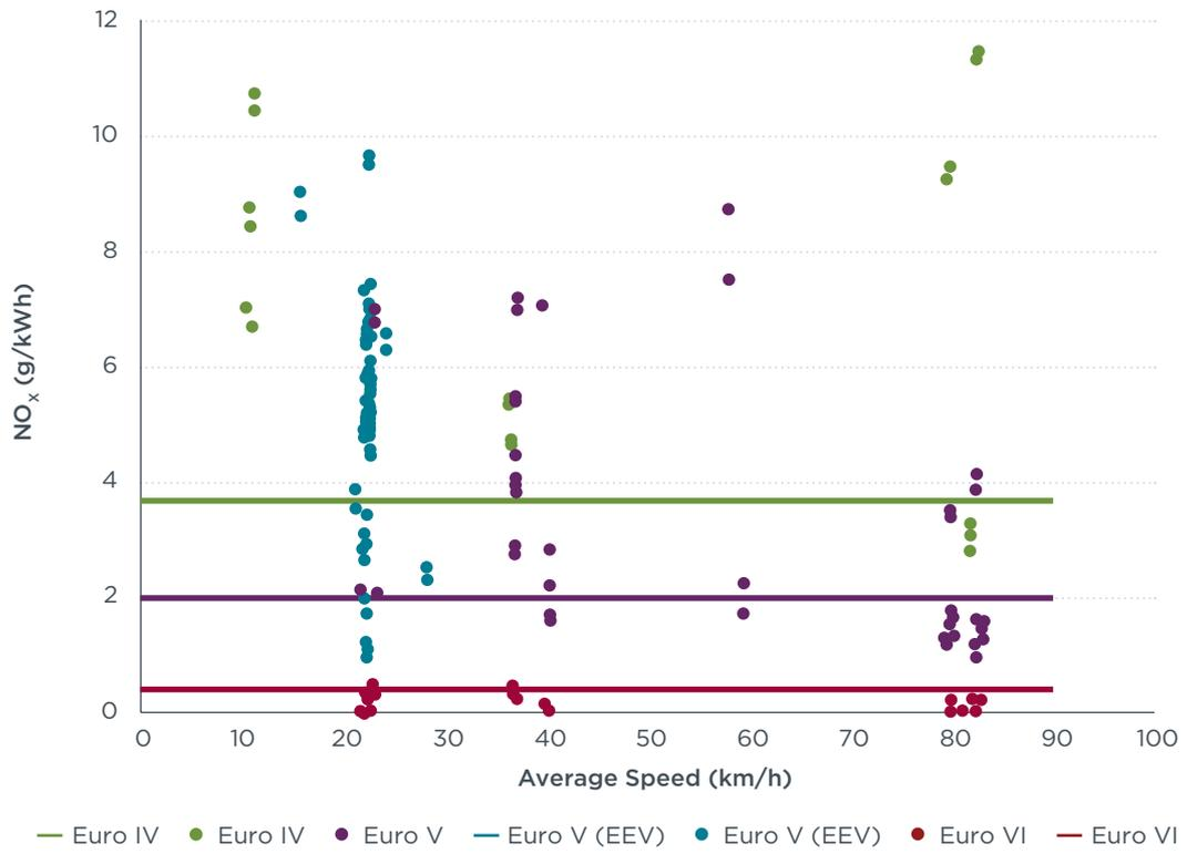
Figure 1. Euro IV, V, VI NO<sub>x</sub> Emissions vs Average Vehicle Speed for all Tests
