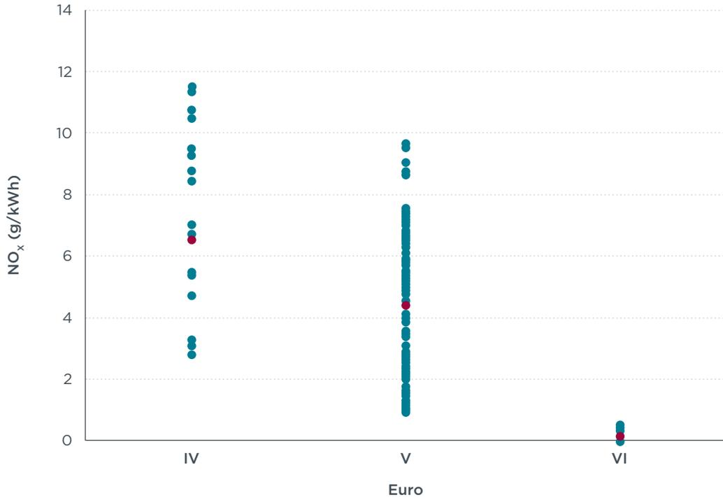
**Figure 3.** NO<sub>x</sub> emissions for all tests plotted vs Euro level. Red point to indicate average of all data
