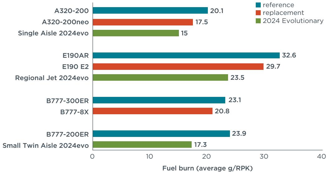
**Figure 7** Fuel burn of reference, emerging successor, and 2024 Evolutionary aircraft
