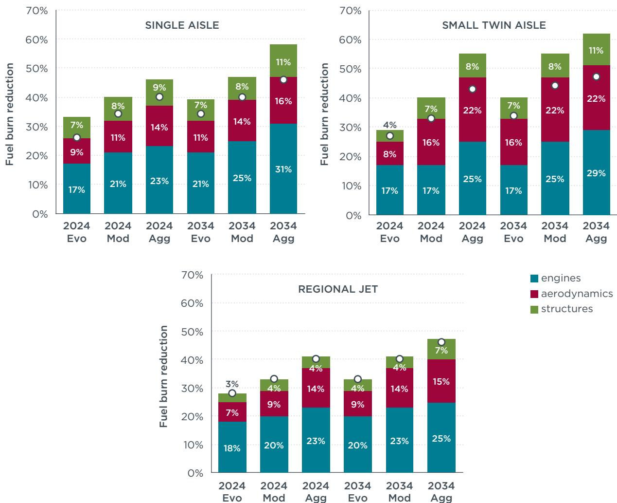
**Figure 6** Fuel burn reductions by aircraft type and technology group
