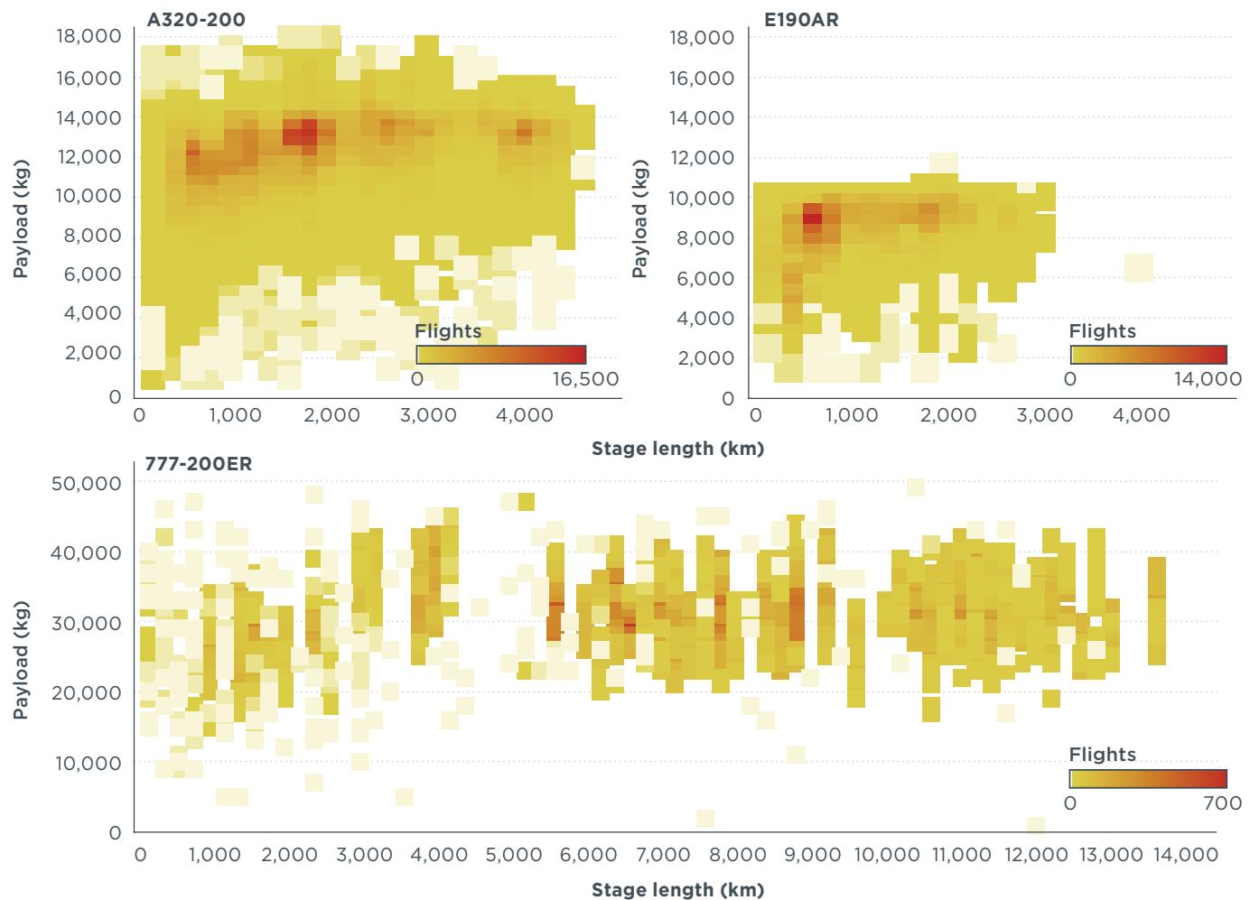
**Figure 4** Typical operations by aircraft type used for fuel burn determination
