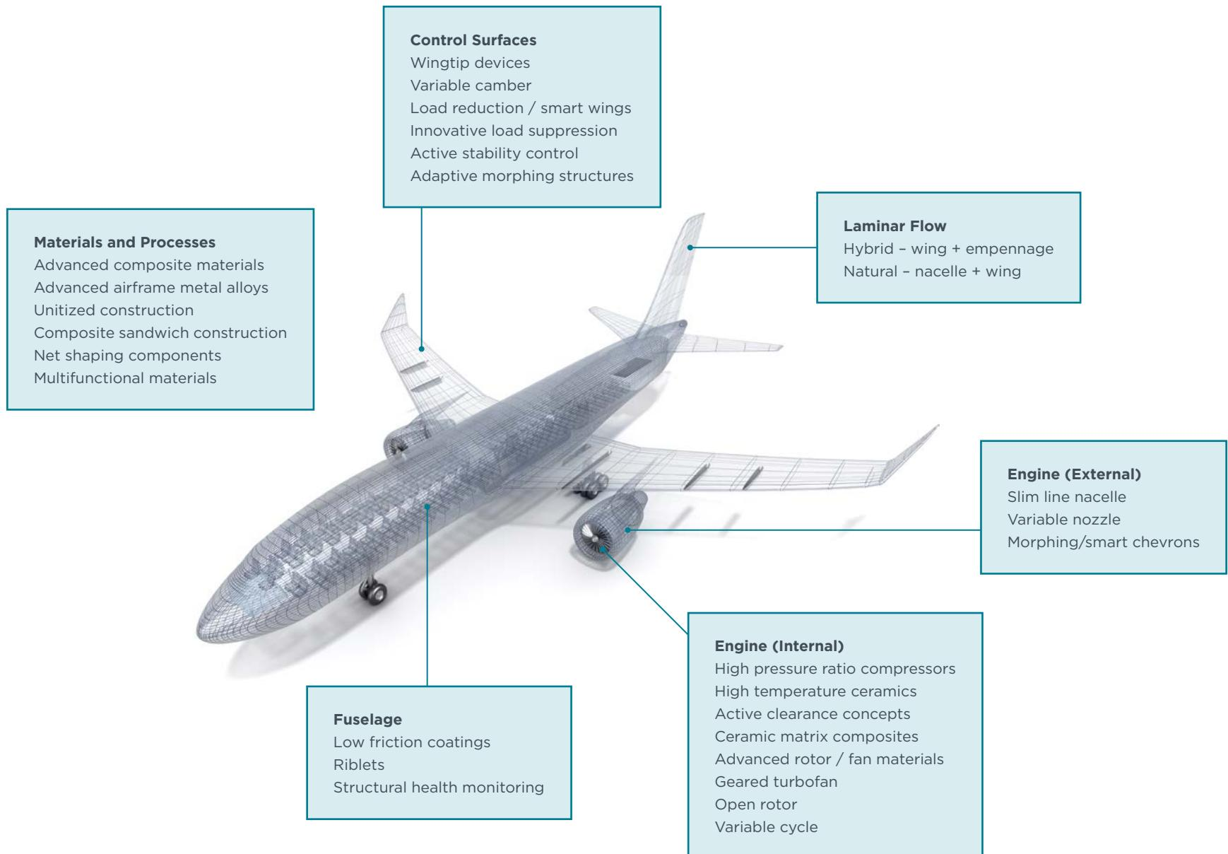
**Figure ES-1** Example aircraft fuel-saving technologies assessed
