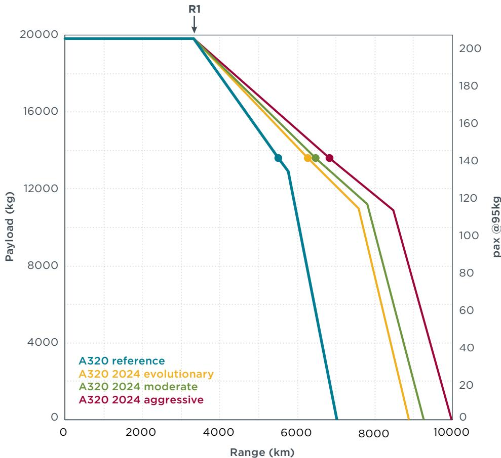
**Figure B 2** Payload-range diagram for single aisle 2024 scenarios
