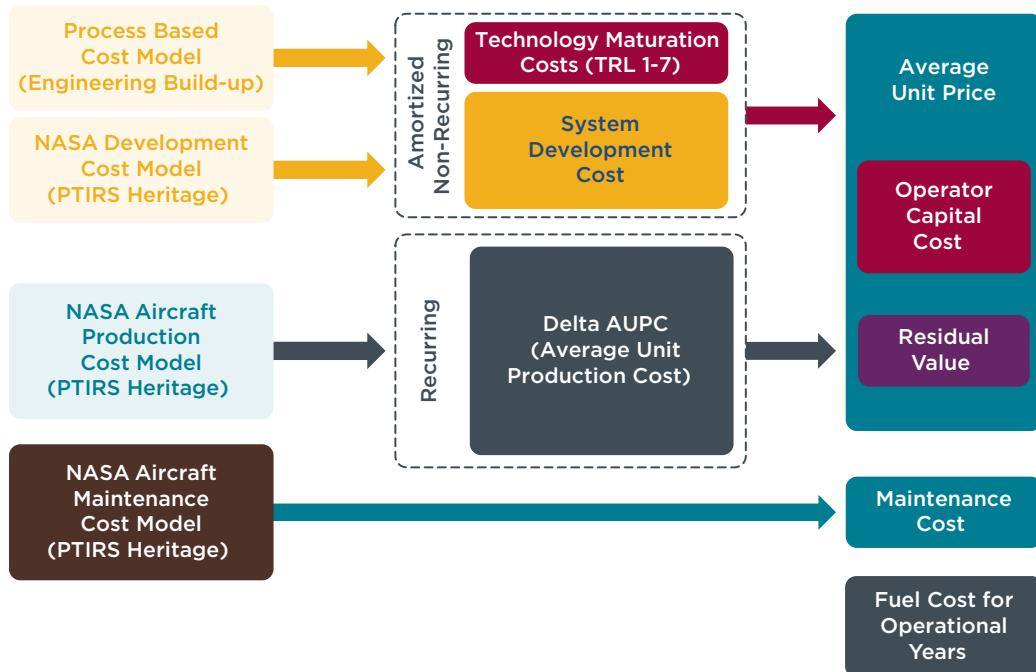
**Figure 5** Total ownership cost determination and components (Tecolote, 2015)
