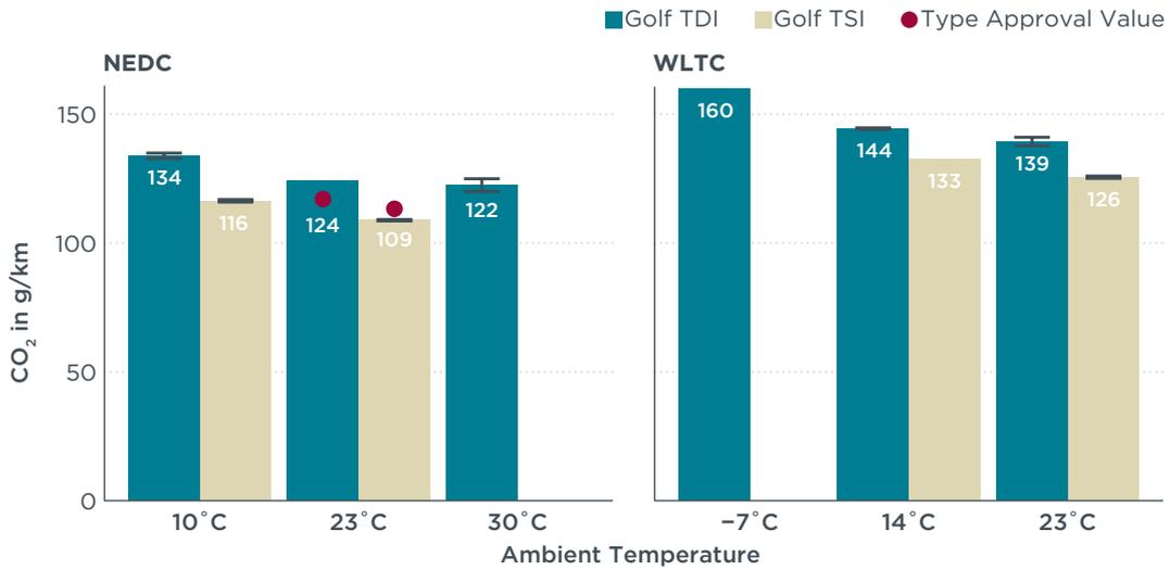
**Figure 6:** Effect of ambient temperature on cold-start WLTC- and NEDC-specific cycle CO<sub>2</sub> emissions. The error bars show the minimum to maximum range of results if multiple tests were performed. No error bar is shown if only one test was performed. The NEDC type-approval emissions are shown with red dots.
