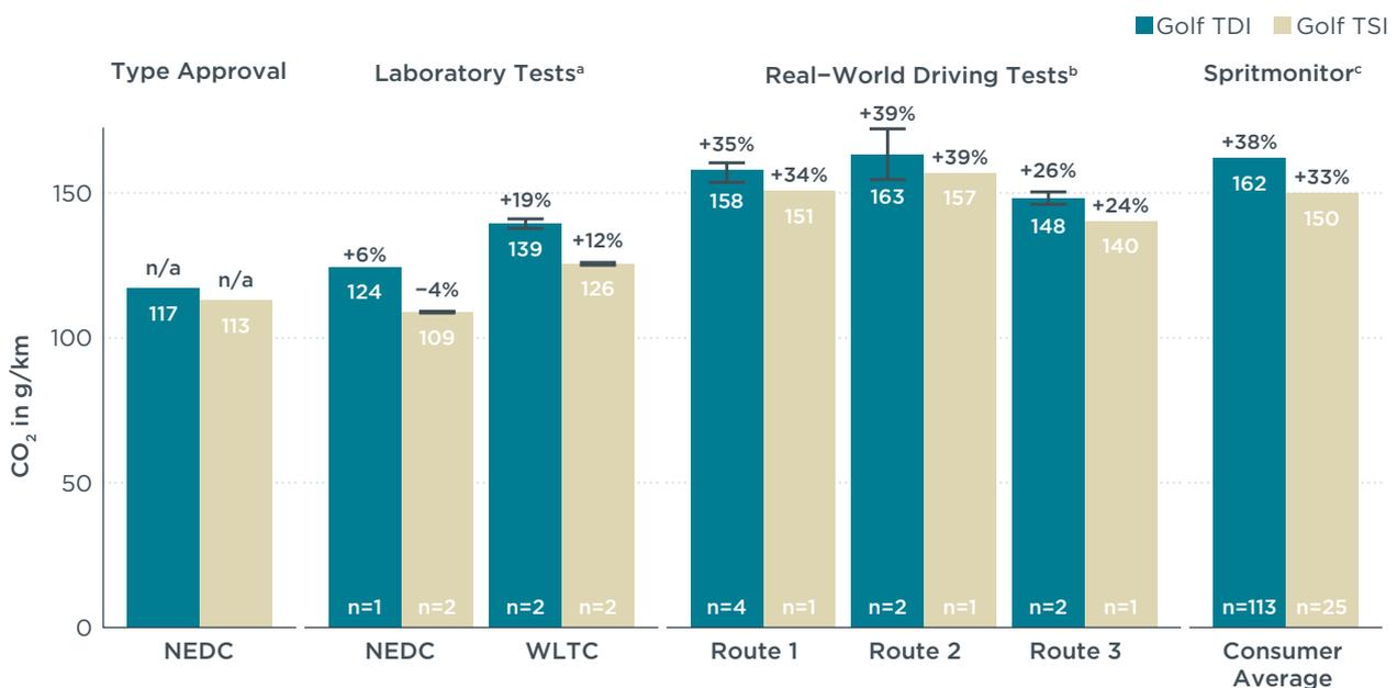
**Figure ES 1.** CO<sub>2</sub> emission levels of the Golf TDI and Golf TSI. Comparison of test results with declared type-approval values and consumer reported numbers (Spritmonitor). The error bars show the minimum to maximum range of results if multiple tests were performed. No error bar is shown if only one test was performed. The number of tests is shown at the bottom of each bar. The relationship of the CO<sub>2</sub> emission level to the type-approval value is shown above each bar.
