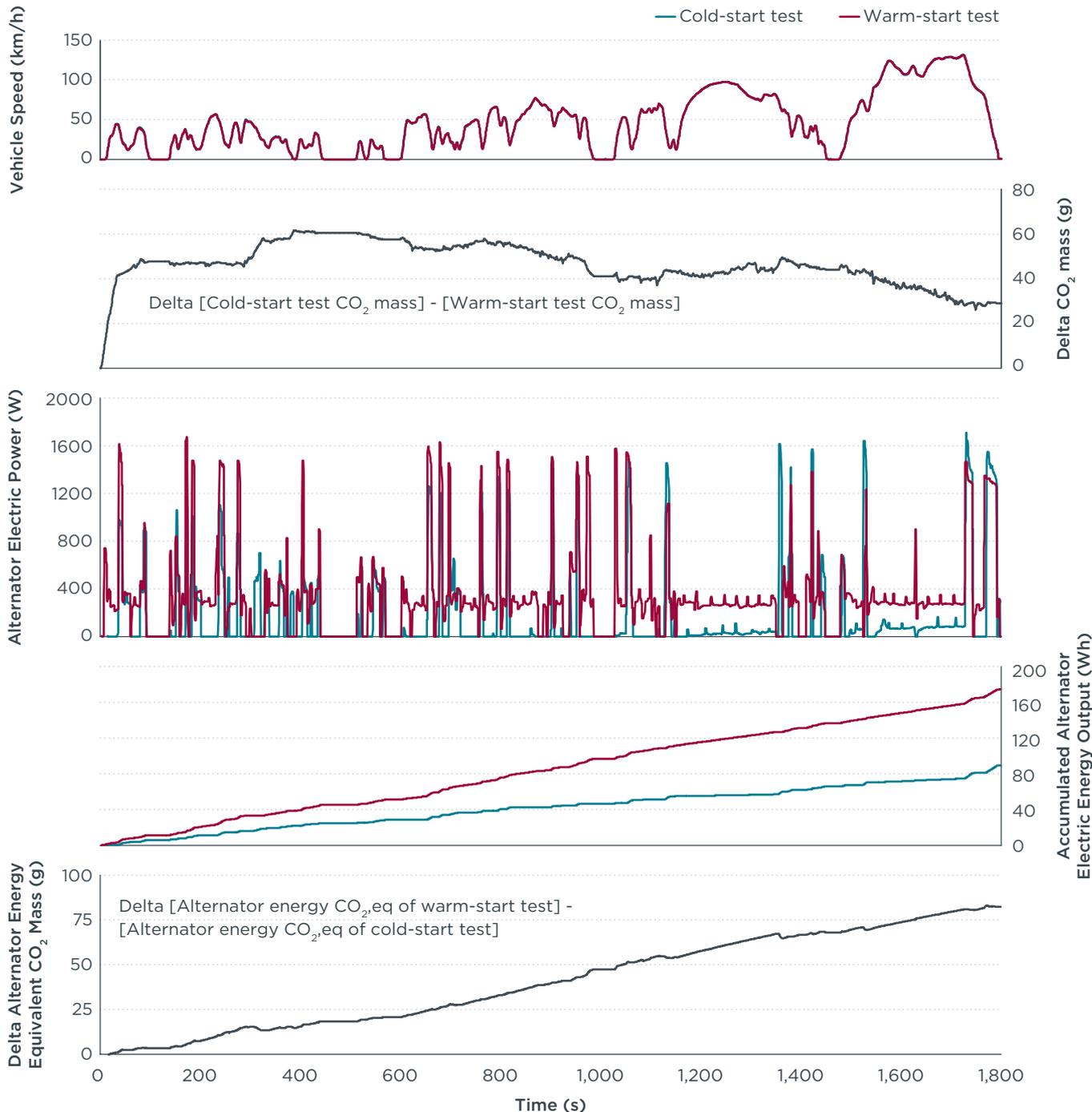
**Figure 12.** Golf TSI alternator power generation in cold- and warm-start WLTC at 23 °C. Alternator energy equivalent CO<sub>2</sub> mass is approximately 82 g higher for the warm-start than for the cold-start test.
