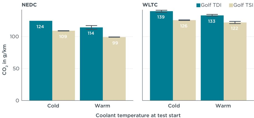
**Figure 7.** Effect of engine coolant temperature at test start on CO<sub>2</sub> emissions—Comparison of Golf TDI and Golf TSI in NEDC and WLTC tests at 23°C. The error bar shows the minimum to maximum range of results if multiple tests were performed. No error bar is shown if only one test was performed.
