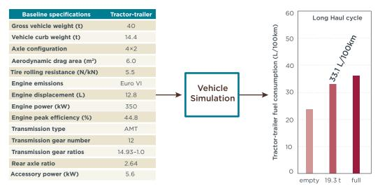
Figure 7. 2015 baseline tractor-trailer for the EU as identified by the ICCT's analysis.<sup>21</sup>
