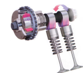
Variable valve controls
