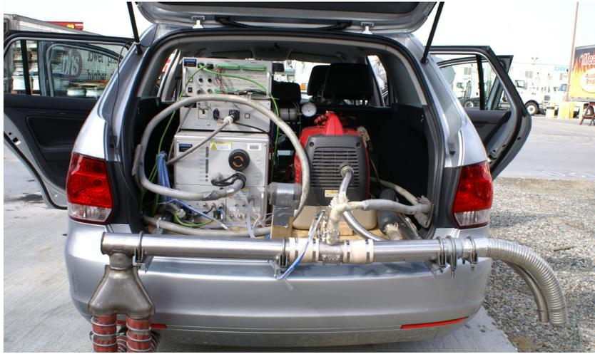
Portable emissions measurement system (PEMS) setup in the Volkswagen Jetta that ICCT had tested as part of the project that eventually led to VW's admission that it had installed defeat devices on 11 million vehicles worldwide.
