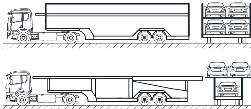
**Figure 33: Violation loading methods of vehicle transport tractor-trailers.**
