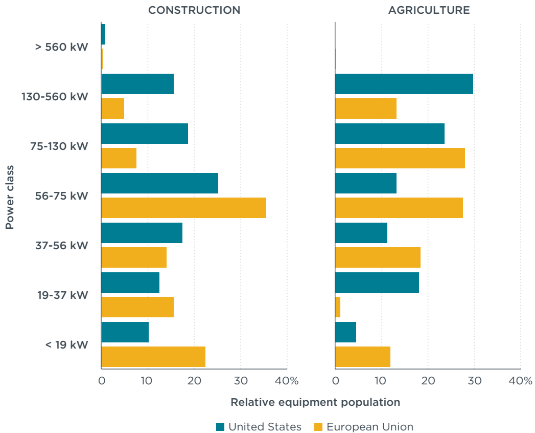
Figure 5. Power class distributions for non-road vehicles and equipment used in construction and agriculture sectors in the United States and European Union (EPA, 2010; EC, 2014a)
