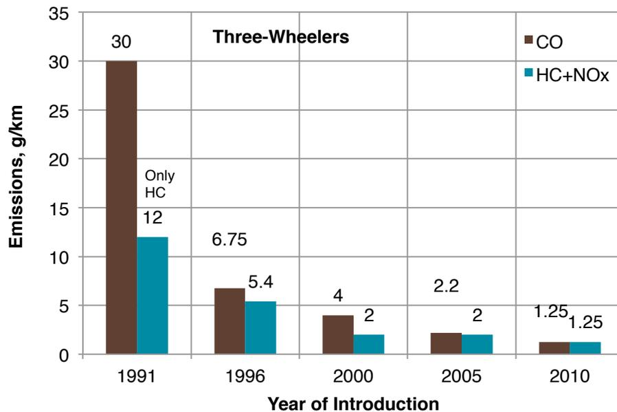
**Figure 21. Progression of Indian Mass Emission Standards for 3-Wheelers (only Spark Ignition Engines)**
