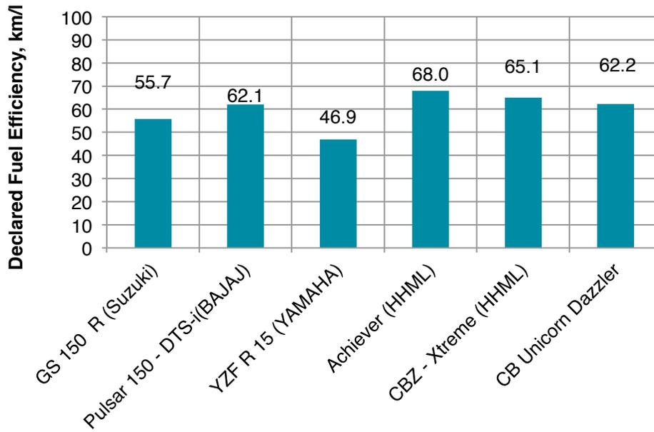
**Figure 38: Comparison of Declared Fuel Efficiency of 150 cc Motorcycles of Different Manufacturers (SIAM 2011)**
