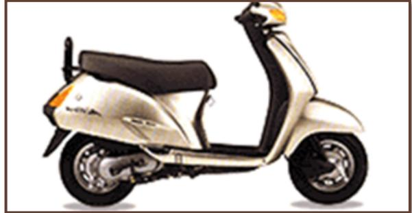
**Scooterettes:** This vehicle is a combination of the moped and the scooter. Its body shape is like that of the scooters but it uses power units, including the transmission, similar to those of the mopeds. It is essentially a low-cost, low-power scooter. They are mostly classified along with scooters.
