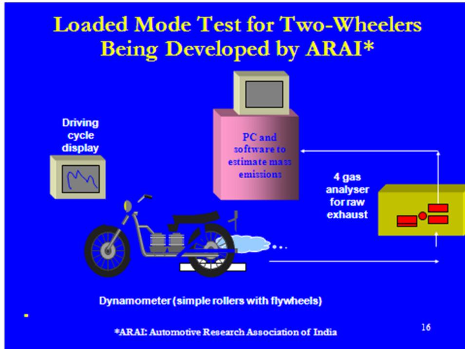
Figure 25: A Schematic Set Up of the Simple Loaded Mode Emission Testing System Developed by ARAI (Courtesy: Automotive Research Association of India)
