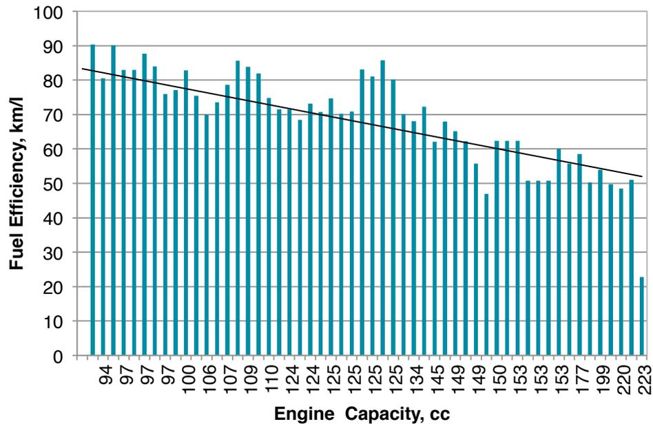
**Figure 35: Declared Fuel Efficiency (km/l) of Motorcycles Related to engine capacity (cc) (all engine capacities)**
