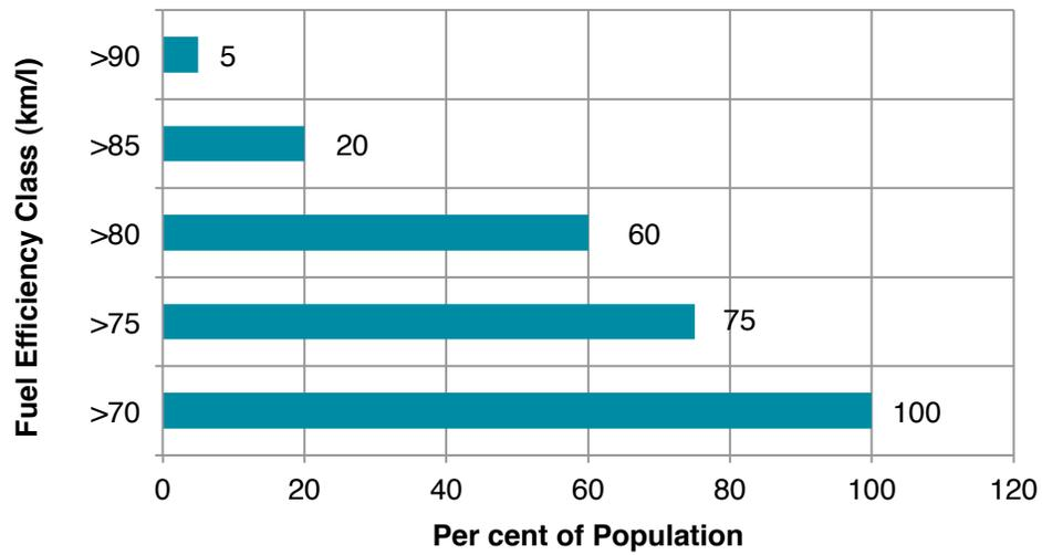
Figure 47: Frequency Distribution of Declared Fuel Efficiency of Motorcycles (75-125 cc), km/l
