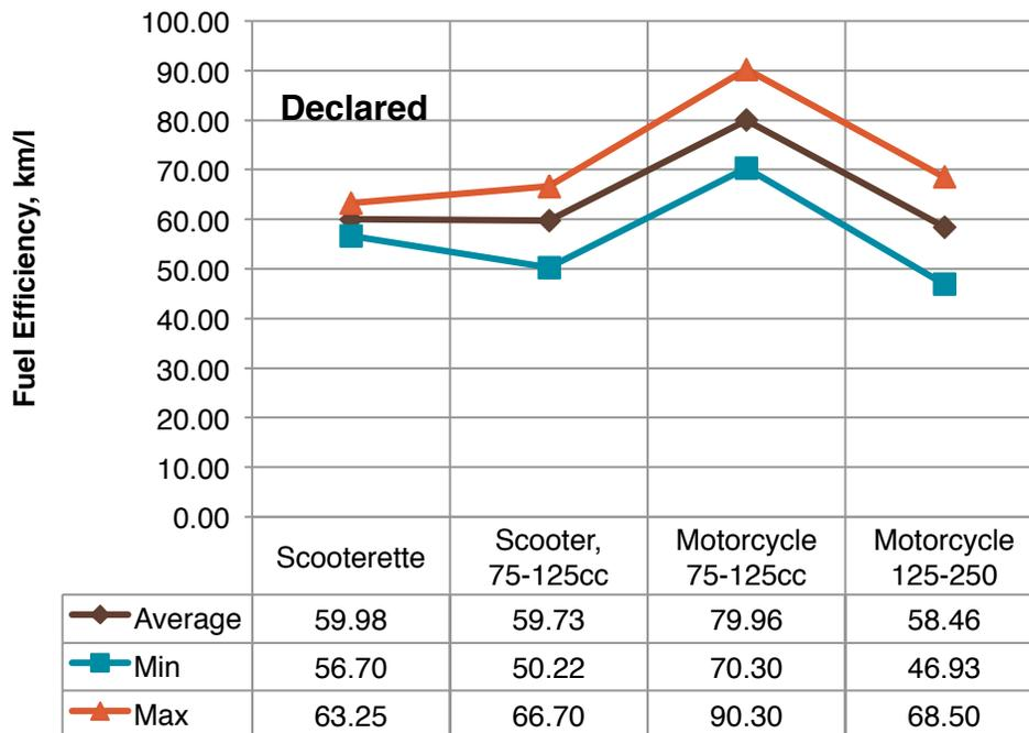
**Figure 31: Range of Declared Fuel Efficiency of Different Categories of 2-Wheelers, (km/l)**
