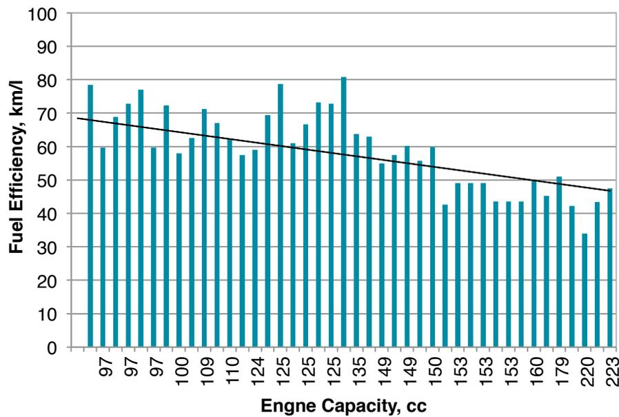
**Figure 36: Reported Fuel Efficiency (km/l) of Motorcycles (all engine capacities) Related to engine capacity (cc)**
