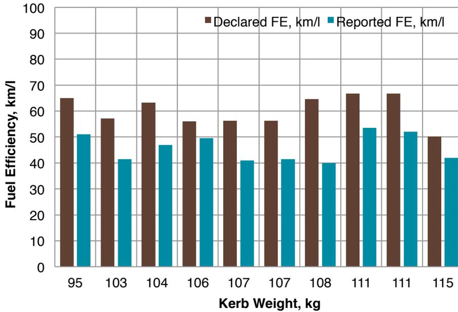
**Figure 39: Relation between Kerb Weight (kg) and Declared and Reported Fuel Efficiency (km/l) of Scooters of 75 to 125 cc.**
