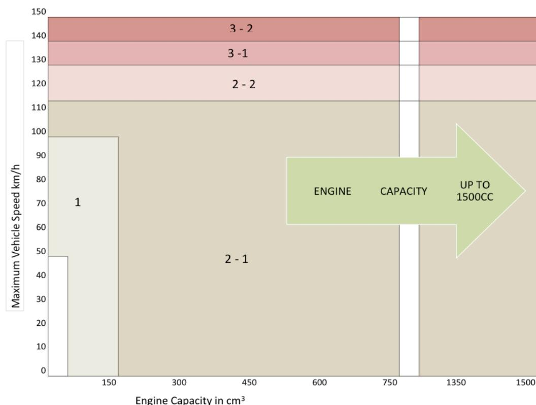
**Figure 22. Diagrammatic Representation of Vehicle Classes Given in GTR2**
