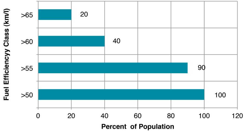
Figure 46: Frequency Distribution of Declared Fuel Efficiency of Scooters (75-125 cc), km/L
