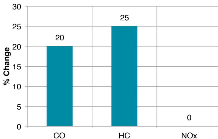
**Figure 24: Results on durability from an 1100 cc Honda Motorcycle. Per Cent Increase in Emissions after 30,000km Test on Honda 1100 cc Motorcycle (*Akamatsu 2004*)**
