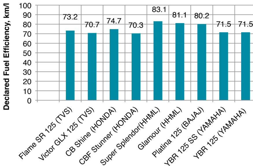
Figure 37: Comparison of Declared Fuel Efficiency of 125 cc Motorcycles of Different Manufacturers (*SIAM 2011*)
