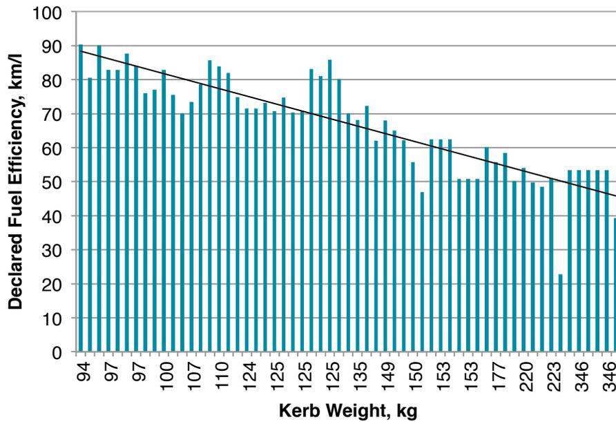
**Figure 40: Relation between Kerb Weight (kg) and Declared Fuel Efficiency (km/l) of Motorcycles (All)**
