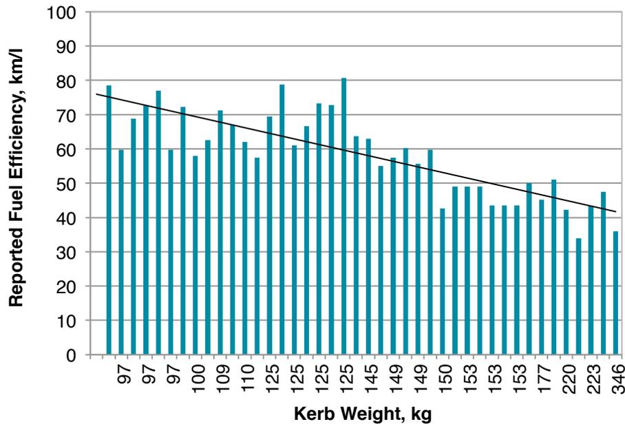
**Figure 41: Relation between Kerb Weight (kg) and Reported Fuel Efficiency (km/l) of Motorcycles (All)**
