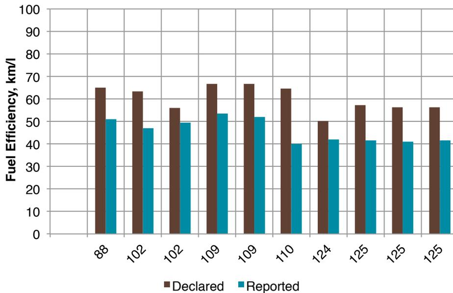
**Figure 34: Declared and Reported Fuel Efficiency (km/l) of Scooters (75-125 cc) Related to Engine Capacity (cc).**
