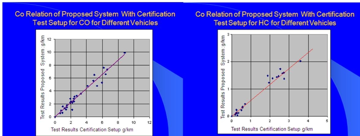
Figure 26: Correlation between the emissions of CO and HC measured on the loaded mode test and the certification testing (Courtesy: Automotive Research Association of India)
