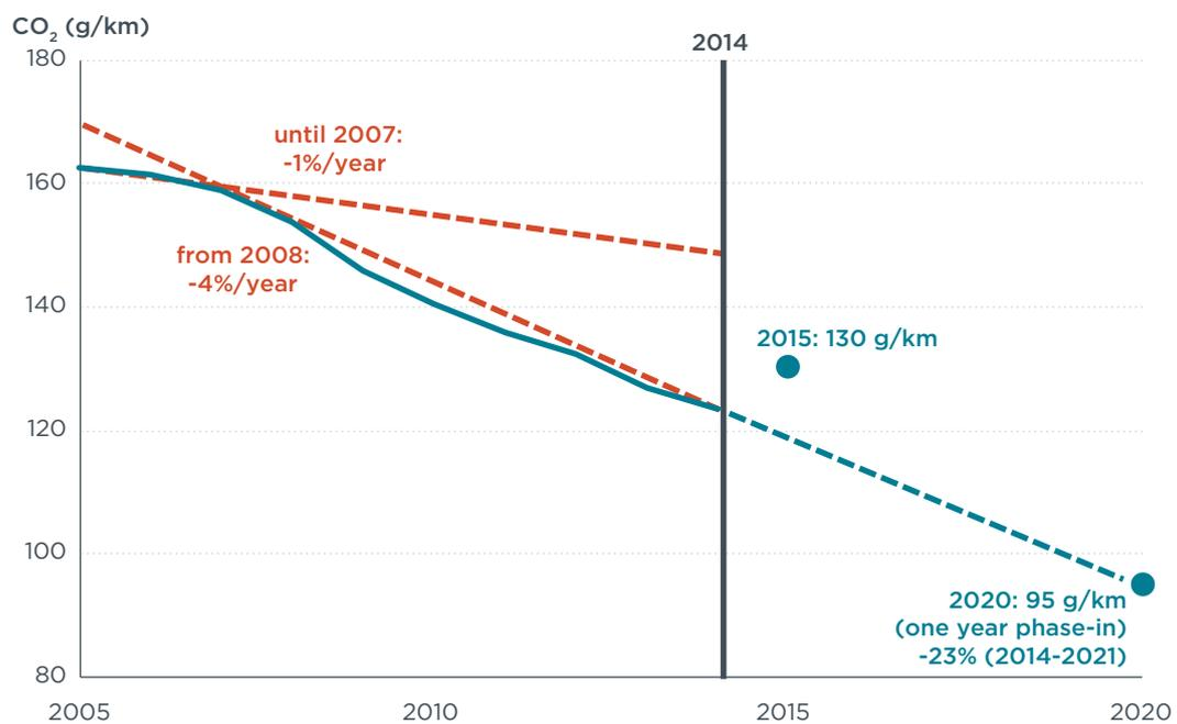
**Figure 1:** Historical development and future targets for CO<sub>2</sub> emission levels of new passenger cars in the EU. Effects of phase-in, super-credits and eco-innovations not shown here.
