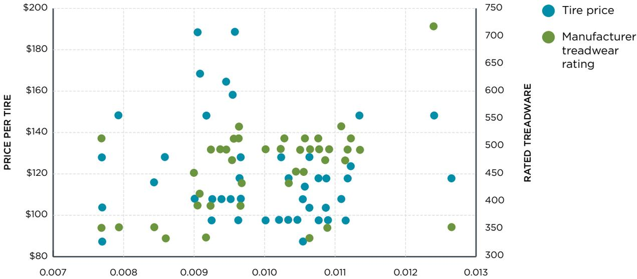
4B. Rolling resistance (tested using JT 609 at 1775 lbs force)
