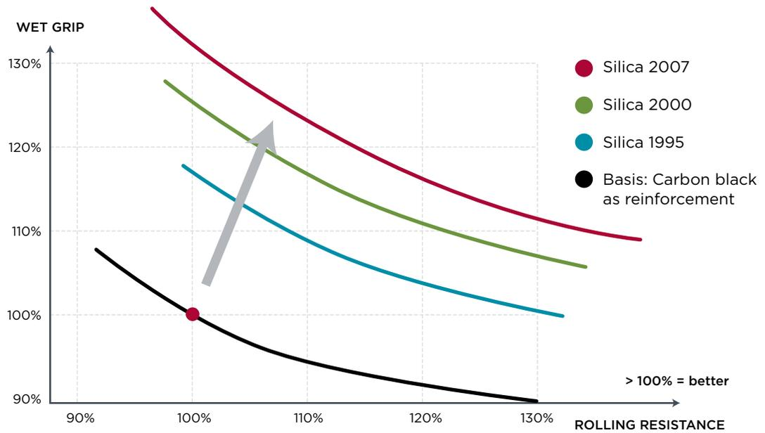
**Figure 3.** Wet grip versus rolling resistance.
