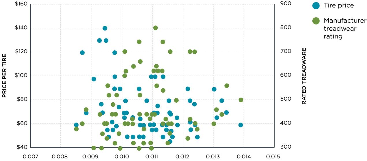
4A. Rolling resistance (tested using JT 609 at 895 lbs force)
