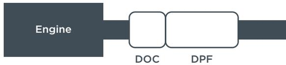
**Figure 5.** DPF system without SCR for US 2007 compliance.
