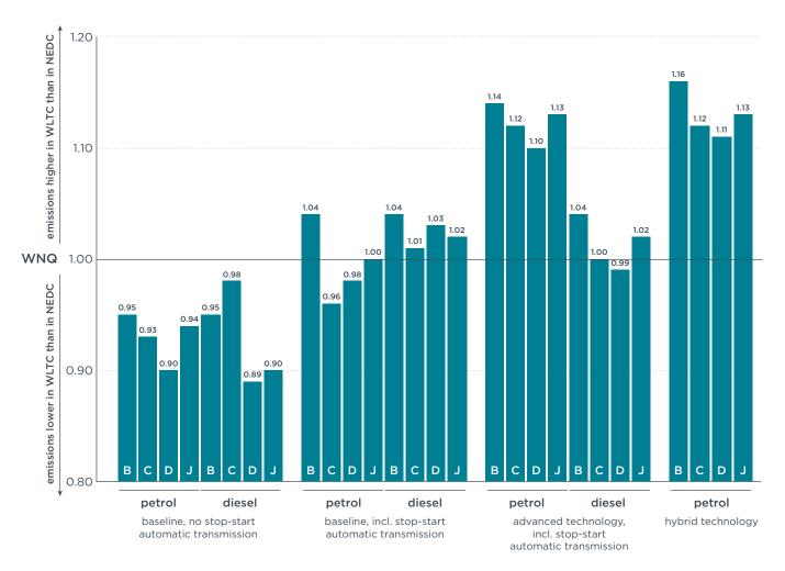
Figure 6. Ricardo vehicle simulations runs and resulting NEDC-WLTC conversion factors
