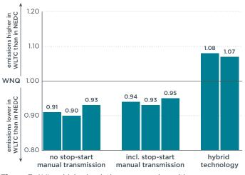
**Figure 7.** AVL vehicle simulations runs and resulting NEDC-WLTC conversion factors
