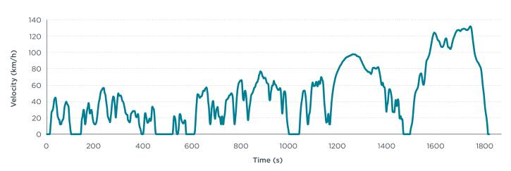
Figure 5. WLTP driving cycle (WLTC)
