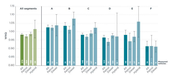
Figure 8. ADAC measurements and derived mean NEDC-WLTC correction factors, broken down by engine technologies and car segments A-F. Error bars represent 95% confidence intervals of the mean WNQs (2x StdDev of the arithmetic mean)
