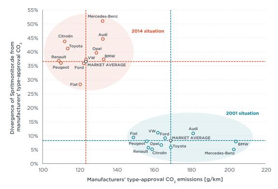
**Figure 32.** Type-approval CO<sub>2</sub> emission values and the corresponding divergence from Spritmonitor.de for selected brands/manufacturers in 2001 and 2014.
