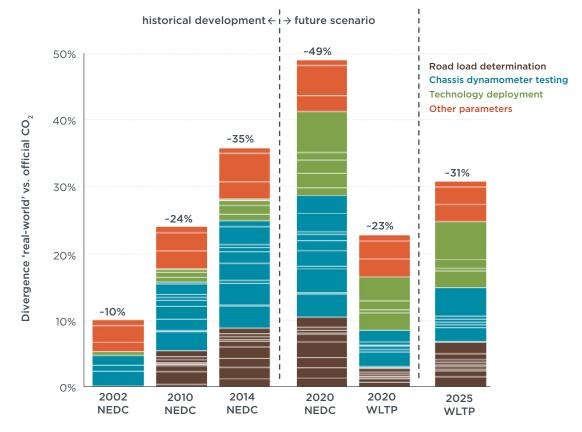
**Figure 2:** Estimate of the reasons for the divergence between type-approval and real-world  $CO_2$  emission levels for new passenger cars in the past as well as in the future, with and without introduction of the WLTP (for details, see Stewart, Hope-Morley, Mock, & Tietge, 2015).
