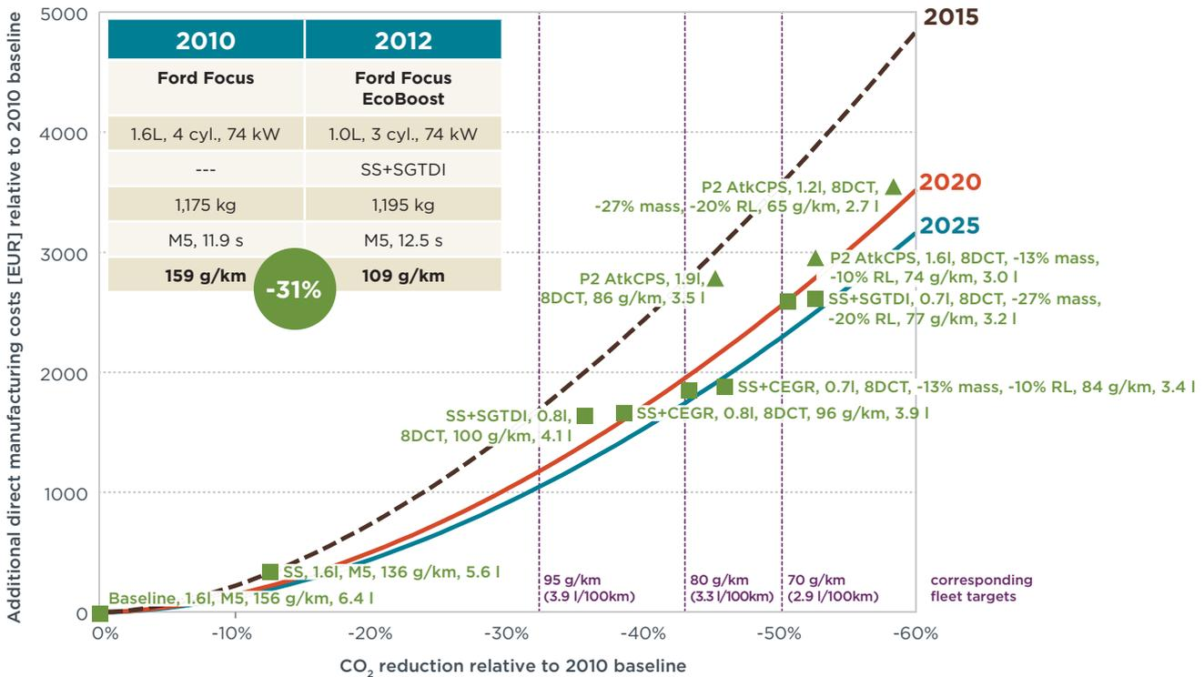
Figure 19. 2012 Ford Focus Compared to C Class Petrol Cost Curve
