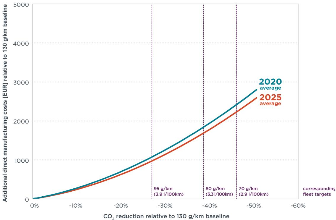
Figure 16. Passenger Vehicle Cost Curves Relative to 2015 EU Target
