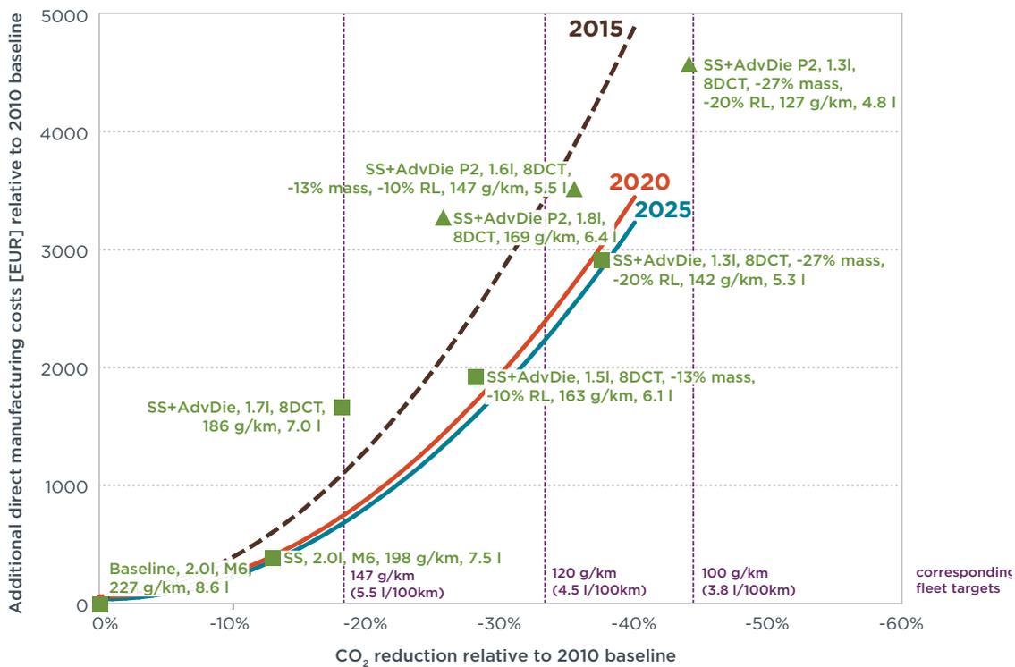
Figure 10. Large N1 Class Cost Curve for Diesel Vehicles
