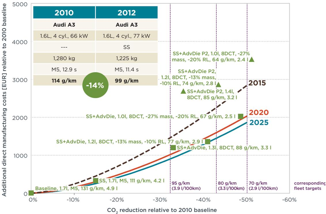
Figure 22. 2012 Audi A3 Compared to C Class Diesel Cost Curve
