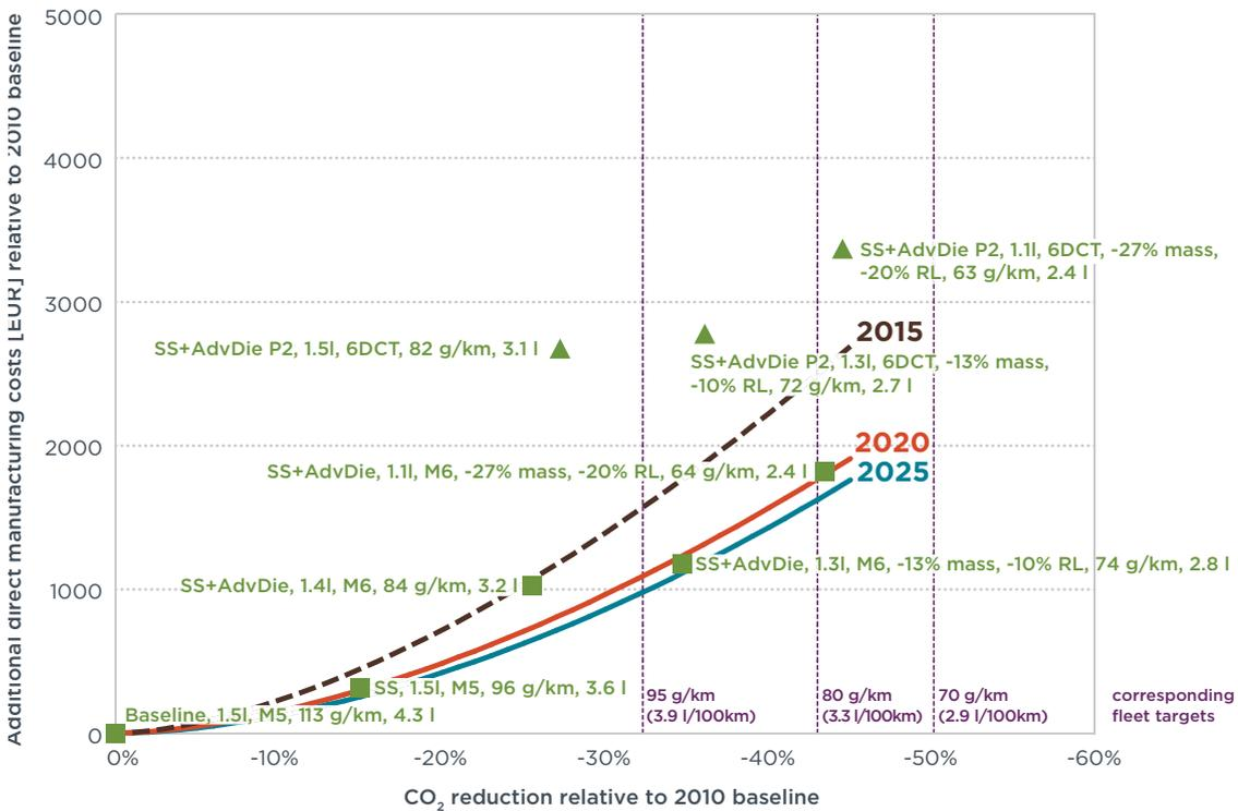
Figure 2. B Class Cost Curve for Diesel Vehicles
