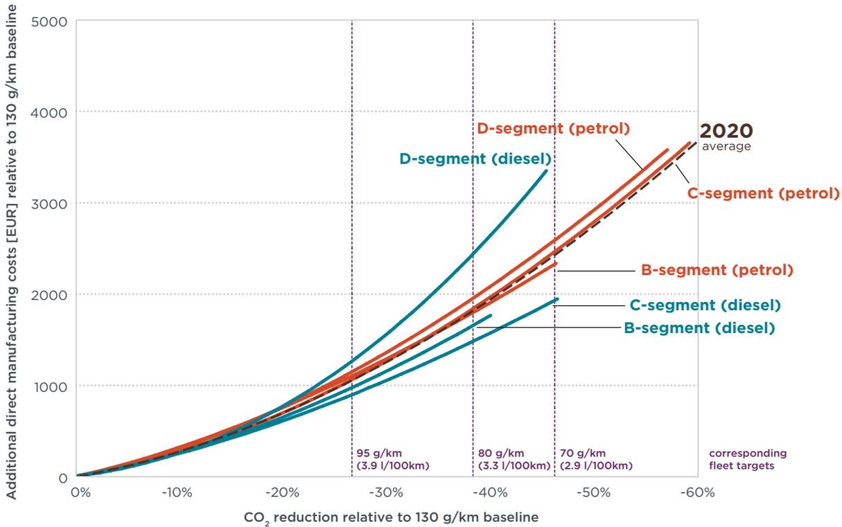
Figure 11. 2020 Passenger Vehicle Cost Curves Relative to 2015 EU Target
