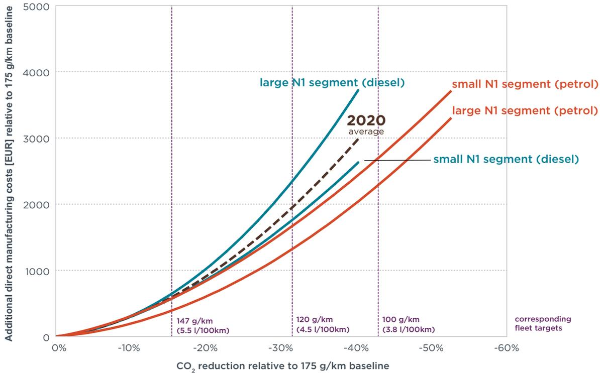
Figure 13. 2020 N1 Class Cost Curves Relative to 2017 EU Target
