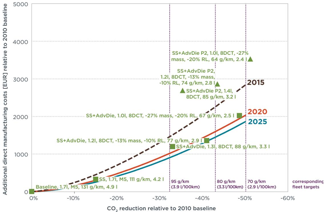
Figure 4. C Class Cost Curve for Diesel Vehicles
