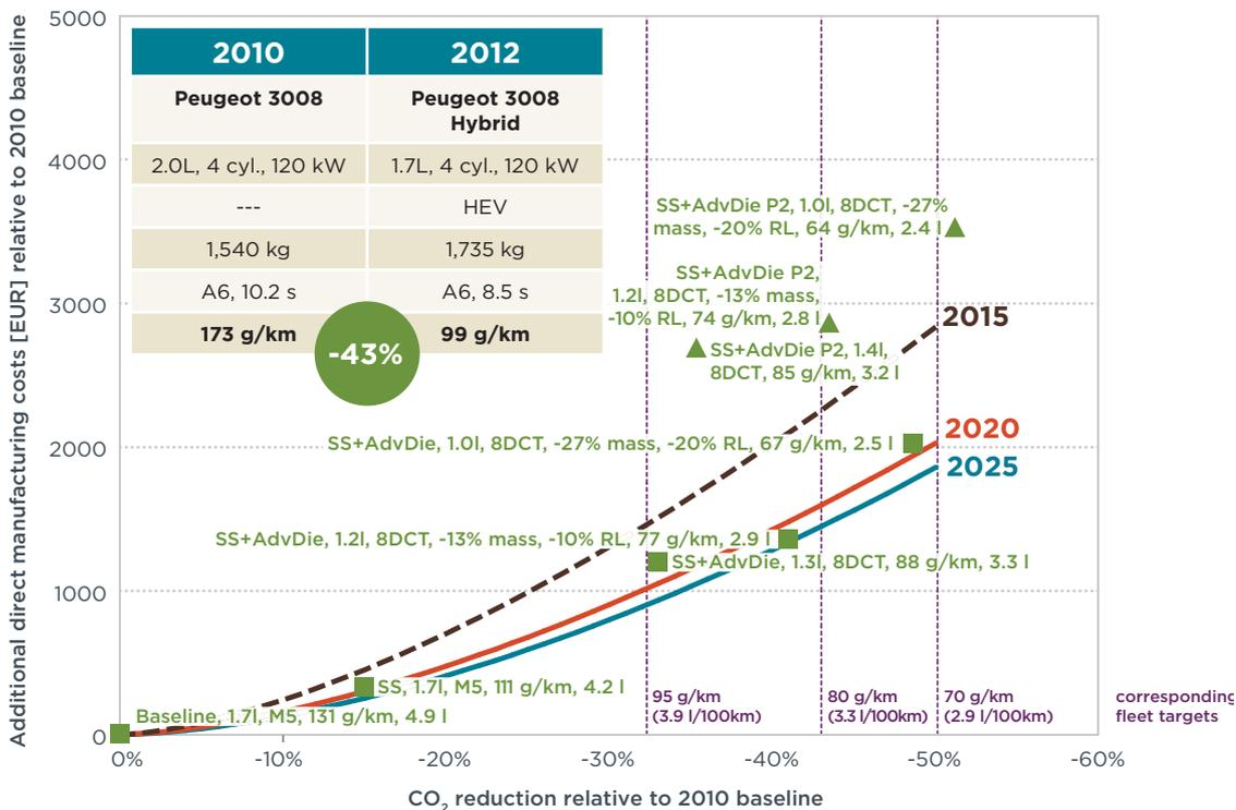
Figure 24. 2012 Peugeot 3008 Compared to C Class Diesel Cost Curve
