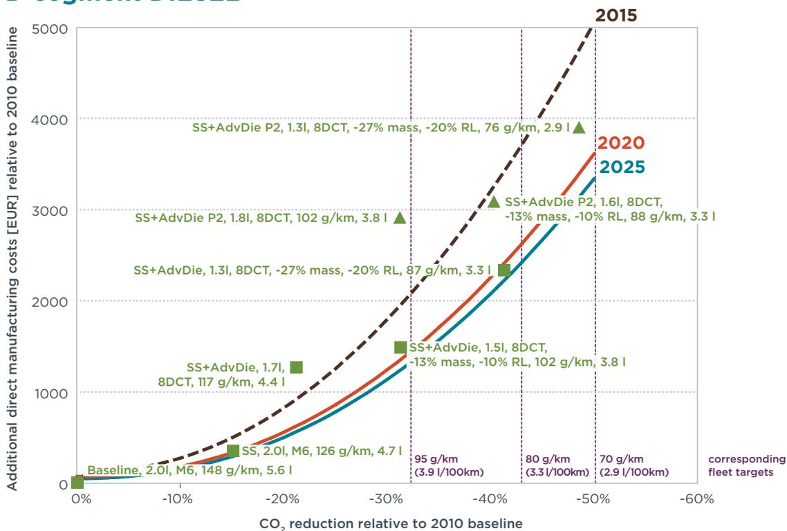
Figure 6. D Class Cost Curve for Diesel Vehicles
