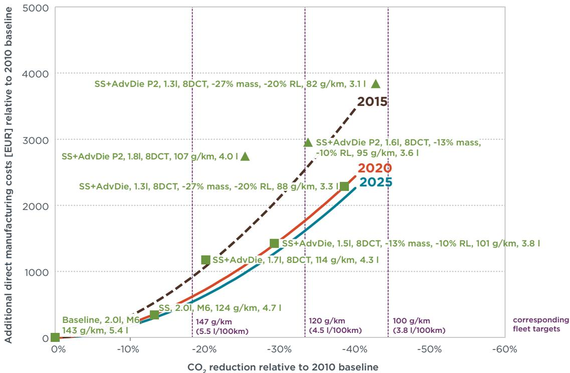
Figure 8. Small N1 Class Cost Curve for Diesel Vehicles
