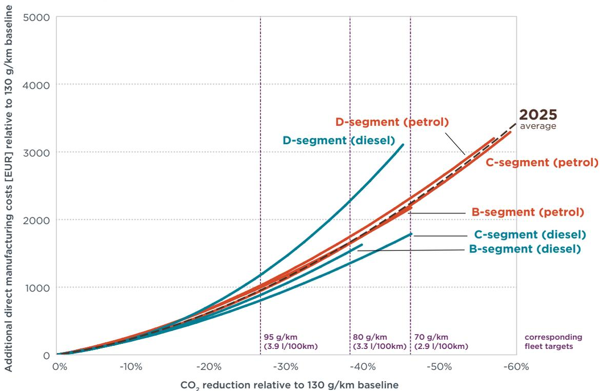
Figure 12. 2025 Passenger Vehicle Cost Curves Relative to 2015 EU Target
