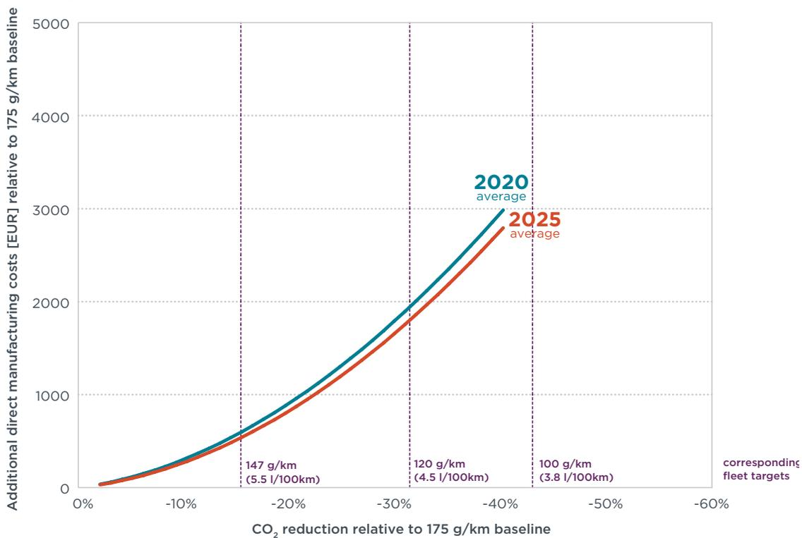
Figure 18. N1 Class Cost Curves Relative to 2017 EU Target
