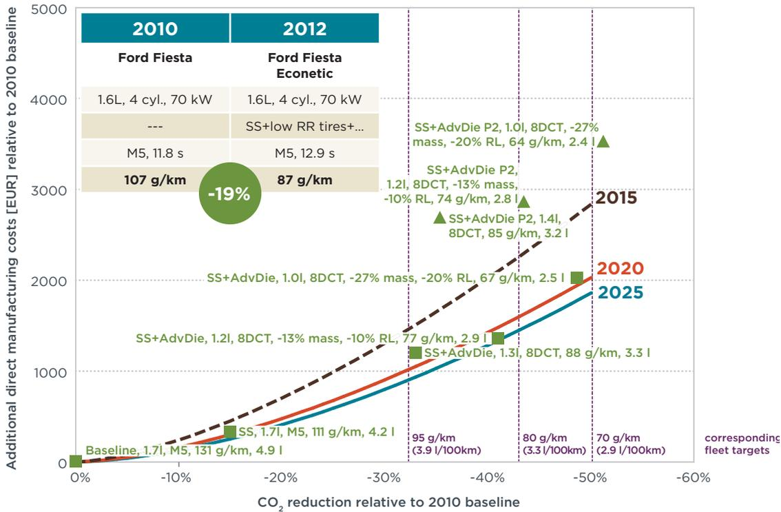
Figure 23. 2012 Ford Fiesta Compared to C Class Diesel Cost Curve
