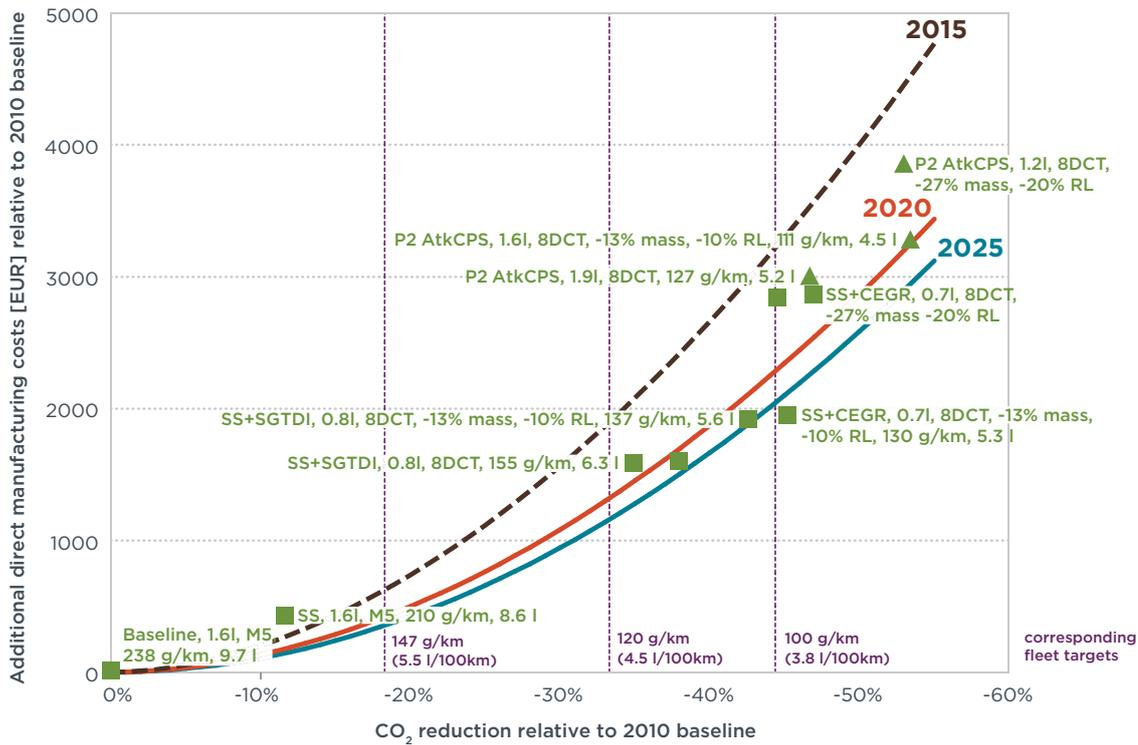
Figure 9. Large N1 Class Cost Curve for Petrol Vehicles
