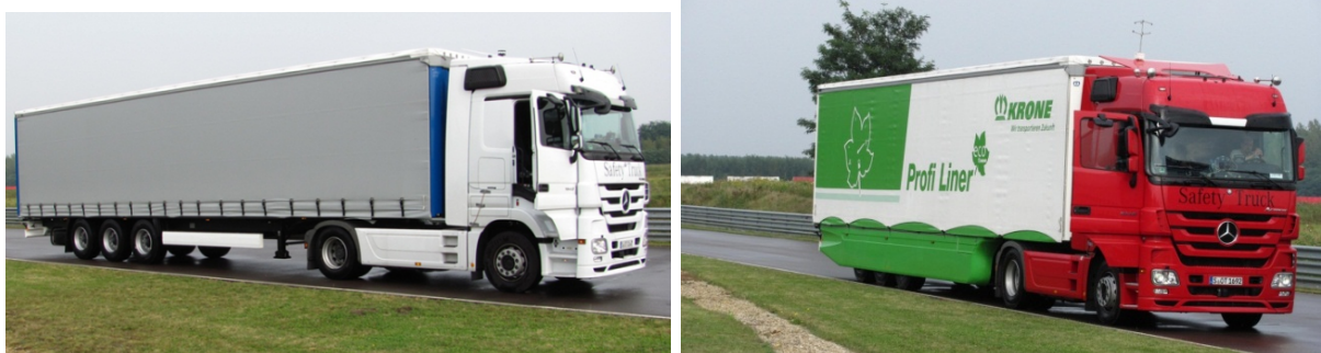
Figure 1: Krone standard trailer and Krone optimized trailer in a 40 ton GVW tractor-trailer combination
