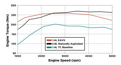
**Figure 10** Torque improvement of EAVS over two baseline engines. (Source: Eaton 2015.)
