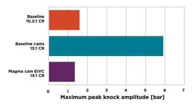
**Figure 8** Comparison of knock amplitude and combustion phasing at 2000 rpm, 20 bar BMEP. (Source: Pendlebury et al. 2016.)
