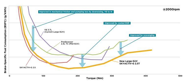
Figure 6 Reduction in fuel consumption of SKYACTIV-G 2.5T at 2000 rpm. (Source: Ichiro Hirose 2016.)
