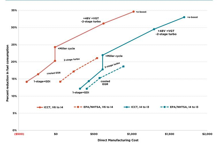
Figure 14 Comparison of ICCT/supplier and EPA/NHTSA costs and benefits of turbocharging and downsizing technologies.
