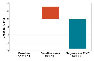
**Figure 9** Comparison of gross ISFC at 2000 rpm, 20 bar BMEP relative to the baseline engine. (Source: Pendlebury et al. 2016.)
