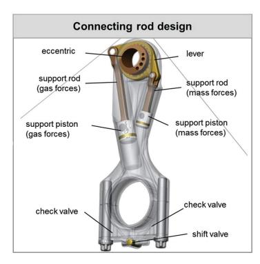
**Figure 11** Two-stage connecting rod design. (Source: FEV 2015 report.)
