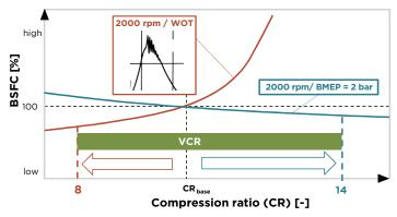
**Figure 12** Fuel consumption dependence on compression ratio under part and full load operation conditions. (Source: Kleeberg, H. et al 2014.<sup>80</sup>)
