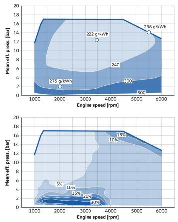
**Figure 5** Top - VW EA 211 1.5-L TSI evo specific fuel consumption engine map. Bottom – Percent reduction in fuel consumption versus baseline turbocharged engine. (Source: Eichler et al. 2016.)
