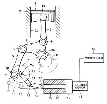
Figure 13 Nissan multi-link system for variable compression ratio<sup>86</sup>
