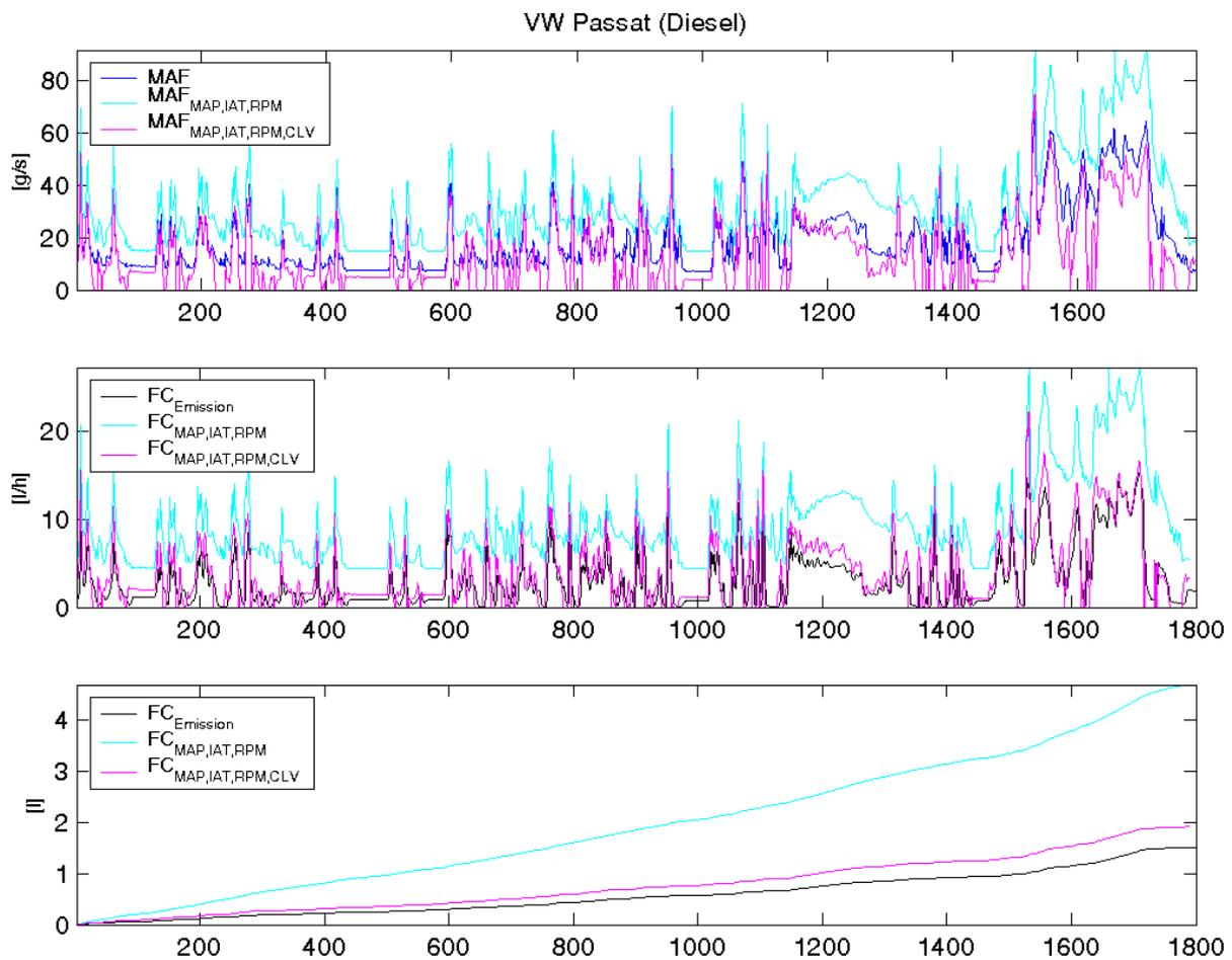
The FC calculation based on the MAF sensor results in values much larger than  $FC_{Emission}$ , but with smaller deviations compared to the MAP based calculation. The product of the MAF and the calculated load results in a curve shape that is much closer to the emission based calculation. Nevertheless, there are deviations in both curve shapes that add up in the total fuel consumption. At higher speeds as seen at around 1600 to 1800 seconds the deviation increases.
