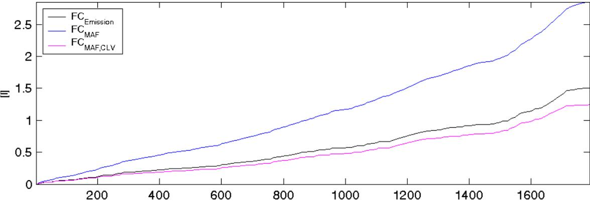
The following diagrams show the emission based calculation of the fuel consumption  $FC_{Dyna}$  against the calculated load value and the manifold air pressure values provided by the vehicle OBD system. Subsequently to the initial experiments of this study, the investigation of further methods for estimating the vehicle fuel consumption based on the CLV could show if the accuracy could be improved, in particular if the vehicle does not support the MAF sensor data.
