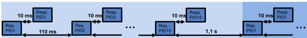
It was observed that the device sends each PID request in a separate CAN message. The vehicle OBD system replies every request after up to 10 ms and it takes more than 110 ms until the device sends the next PID request in a CAN message. After all 15 PIDs are requested the device waits around 1 second until the next read cycle starts. Thus, the time between two requests of the same PID is around 3 seconds.
