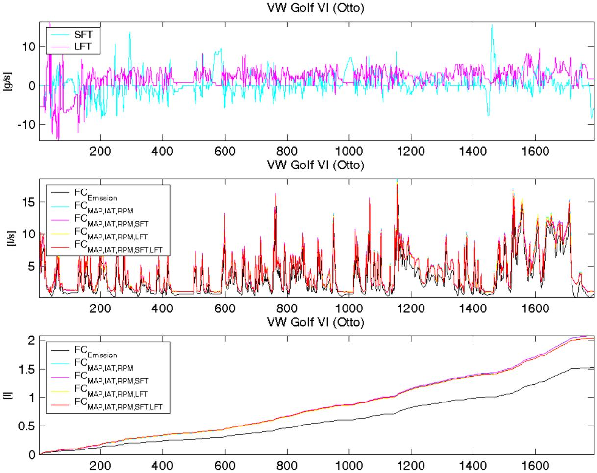
The following diagrams show the emission based calculation of the fuel consumption  $FC_{Dyna}$  against the calculated load value and the manifold air pressure values provided by the vehicle OBD system. Subsequently to the initial experiments of this study, the investigation of further methods for estimating the vehicle fuel consumption based on the CLV could show if the accuracy could be improved, in particular if the vehicle does not support the MAF sensor data.
