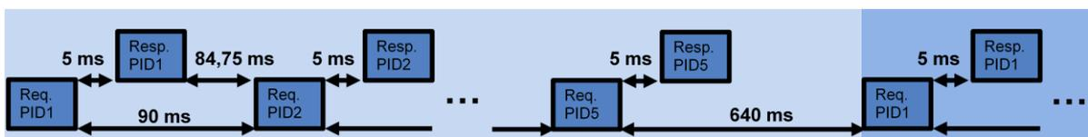
It was observed that the device sends each PID request message in a separate CAN message. For testing device two, a different vehicle was used as for testing device 1. The vehicle OBD system in testing device 2 replies every request after around 5 ms and the device starts transmission of the next PID request message after around 90 ms, which is 40 ms more than the OBD specified maximum value for P2 of 50 ms.
