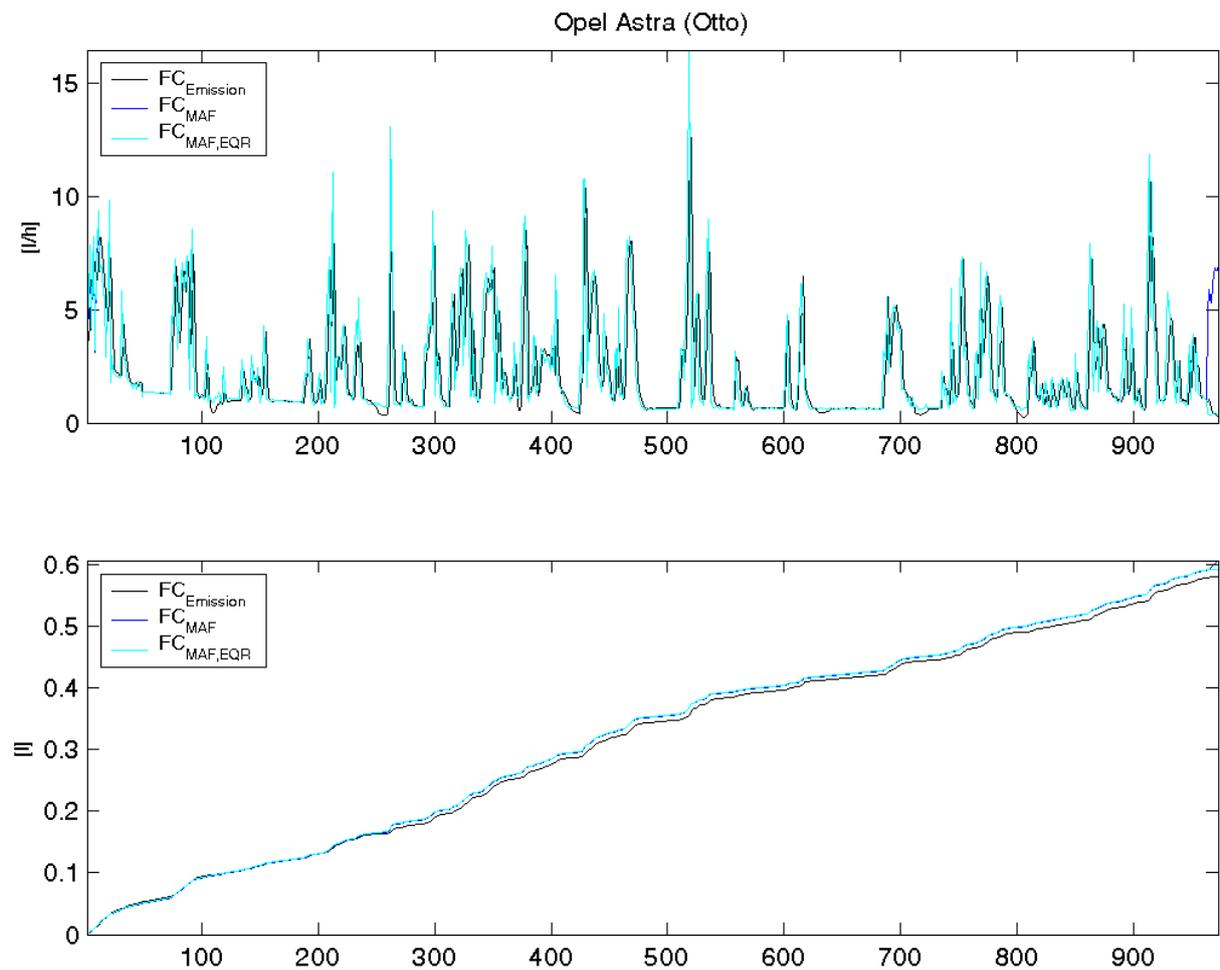
The following diagrams show the emission based calculation of the fuel consumption  $FC_{\text{Dyno}}$  against the calculated load value and the manifold air pressure values provided by the vehicle OBD system. Subsequently to the initial experiments of this study, the investigation of further methods for estimating the vehicle fuel consumption based on the CLV could show if the accuracy could be improved, in particular if the vehicle does not support the MAF sensor data.
