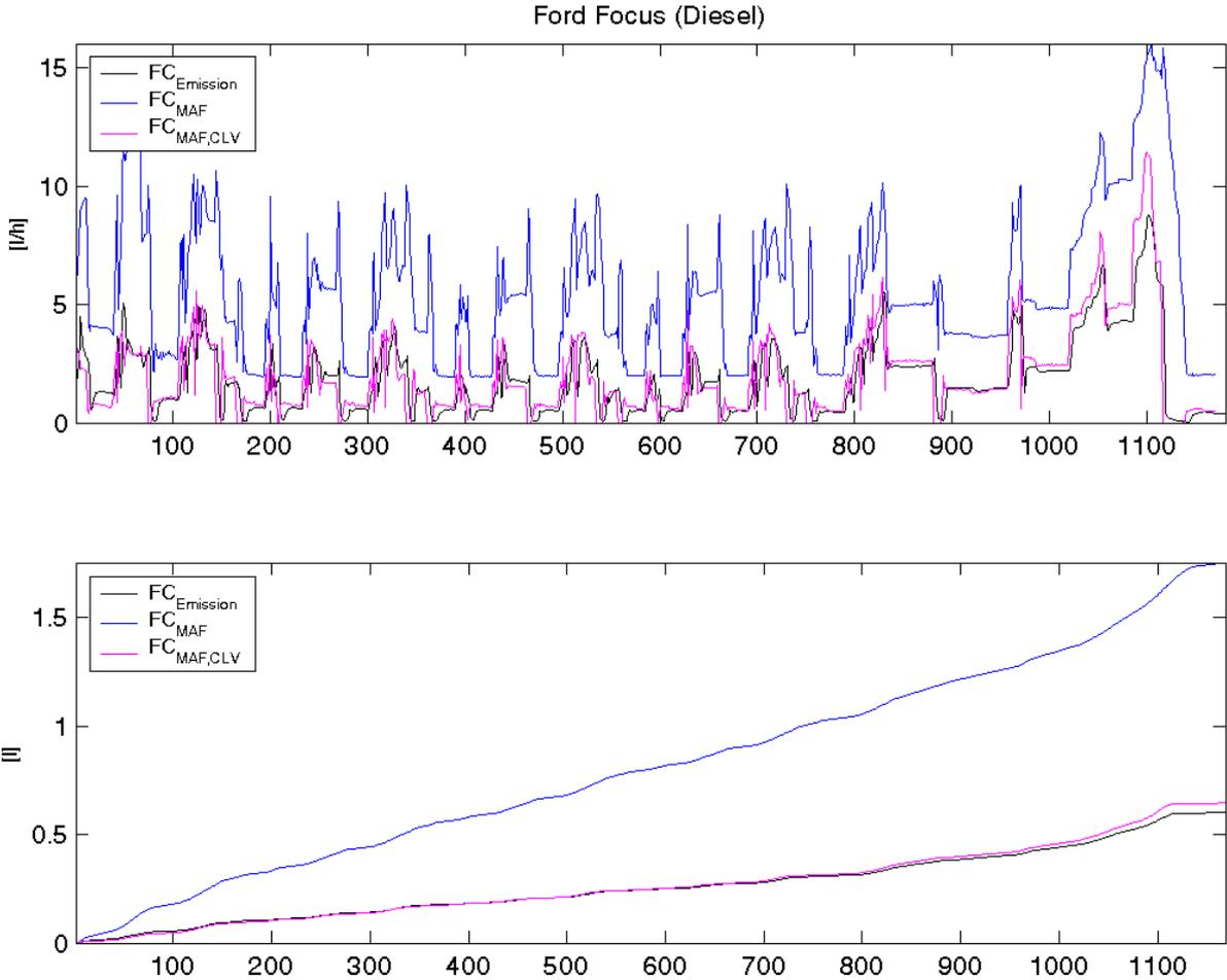
The following diagrams show the emission based calculation of the fuel consumption  $FC_{Dyna}$  against the calculated load value and the manifold air pressure values provided by the vehicle OBD system. Subsequently to the initial experiments of this study, the investigation of further methods for estimating the vehicle fuel consumption based on the CLV could show if the accuracy could be improved, in particular if the vehicle does not support the MAF sensor data.
