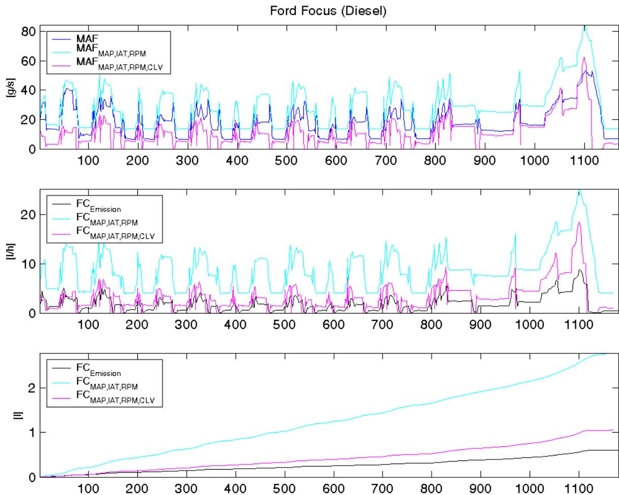
The calculation based on the MAF sensor leads to a much larger values compared to the emission based calculation. But, considering the calculated load value results in a curve shape that is very close to the emission based calculation, although at higher speeds the deviation increases. The curves of the total fuel consumption in liters show a very good matching especially at speeds below 100 km/h.
