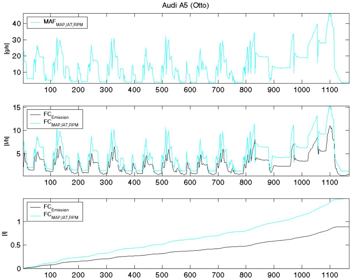
The experiment to improve the  $FC_{MAP,IAT,RPM}$  results with consideration of the long term and short term fuel trim values are visualized in the following diagrams. SFT and LFT modify the air-to-fuel ratio over time, which is set to the constant value of 14.7:1. The plots of the  $FC_{OBD}$  values with different combinations of SFT and LFT show only marginal improvements compared to the deviation to the  $FC_{Dyno}$  curve.
