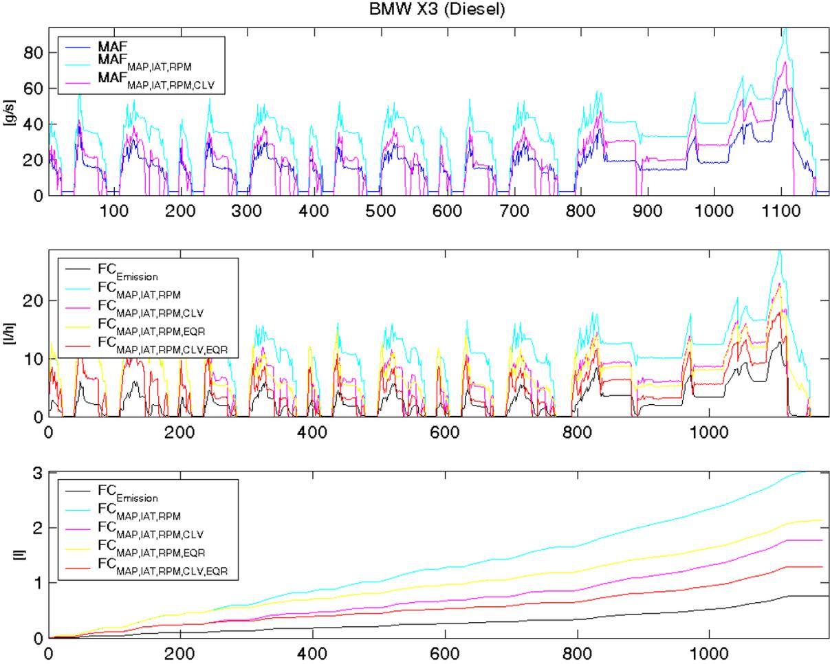
Similar to the results from the other vehicle measurements the calculation based on the MAF sensor leads to a higher accuracy when considering the calculated load value. The deviation of the total fuel consumption to  $FC_{Emission}$  is similar to the Ford Focus vehicle measurements but in the opposite direction. While  $FC_{MAF}$  is lower than  $FC_{Emission}$  for the Ford Focus, it is higher for the BMW.
