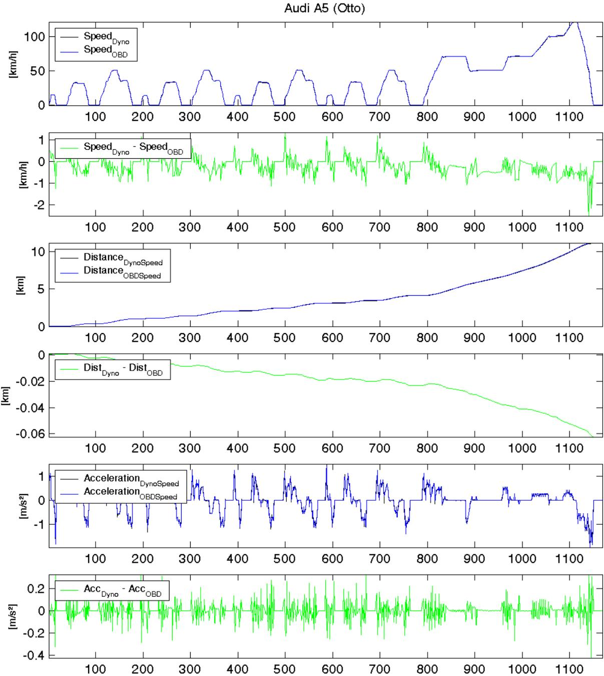
As the deviations in the range of +/-1 km/h are relatively small and also compensate over the whole driving cycle, the calculated distance does not show considerable deviations. Nevertheless the deviations influence the calculation of the total fuel consumption.
