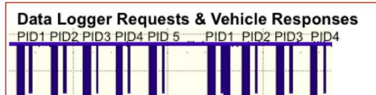
For the K-Line protocols each PID has to be requested within an individual message. The messages transmitted by the data logger have a specified length of 6 byte with an inter-byte time of around 6 ms. Therefore each individual PID request has a transmission length of around 36 ms. In the test, the vehicle wait time P2 between the request and the single ECU vehicle response is around 30 ms and the single ECU vehicle response has a length of around 7 ms.
