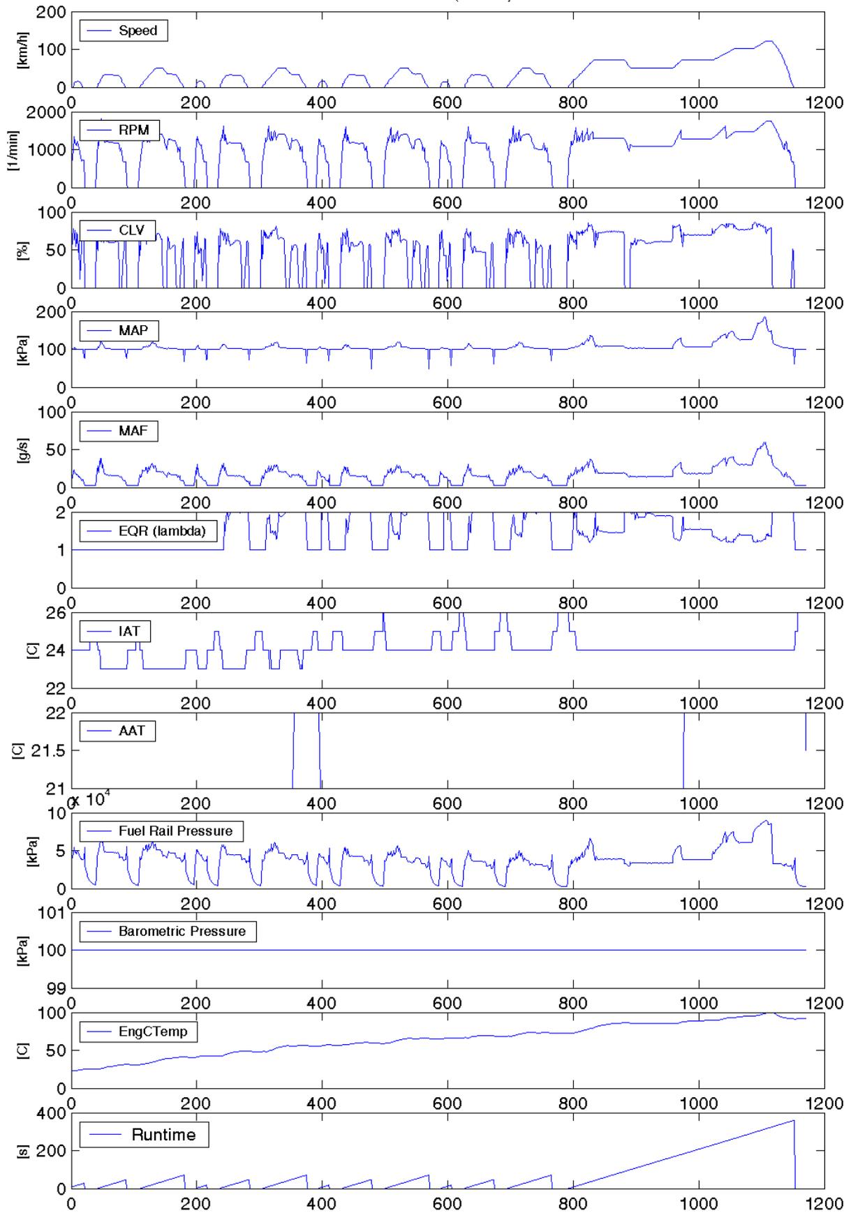
The comparison of the measured speed values shows that the deviations of the OBD and the Dyno measurement lies in the range of +/-2 km/h in the lower speed area and increase up to -3 km/h at 120 km/h. The calculated distances show only low deviations, but would presumably increase on longer distances at higher speeds.
