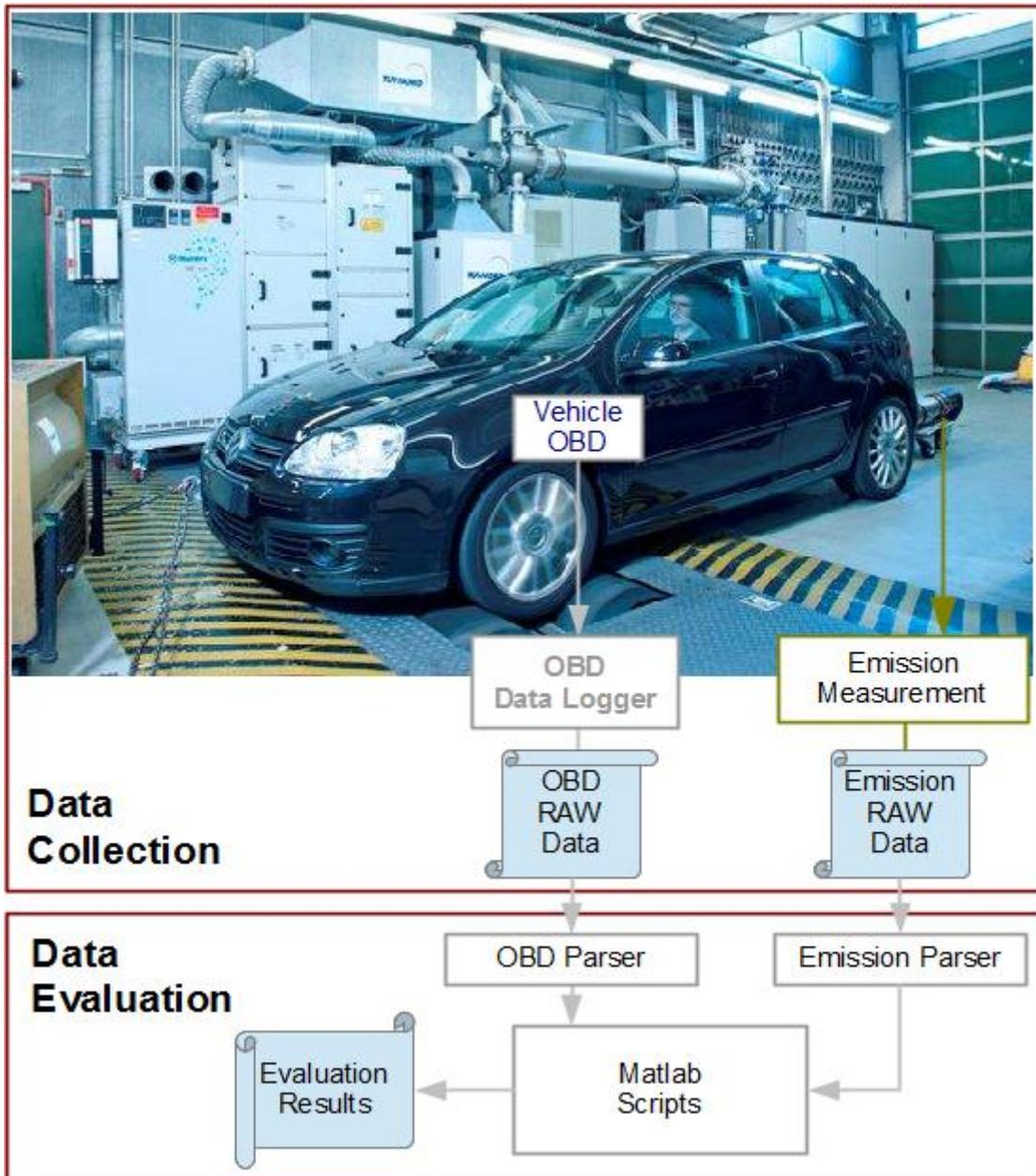
The measurement equipment delivers a record-file containing masses of the vehicle emission pollutants (HC, HC<sub>Diesel</sub>, CH<sub>4</sub>, NOX, NO, CO, CO<sub>2</sub>) given in milligram per second as well as the corresponding vehicle speed in kilometers per hour and the power given in Newton. Based on these measurement values the vehicle fuel consumption was calculated according to the equations given in [ECE\_R101]:
