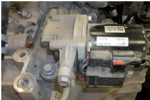
Image 4 (Left): Chevy Malibu auxiliary pump (Source: FEV Library)
